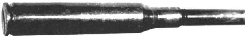
Figure 2-8 - Photograph of the modified 270 case with a 1/4 inch OD steel tube attached for measuring pressure during calibration. The 1/4 inch tube extends down the bore and out the muzzle where it is attached to the hydraulic cylinder shown in Figure 2-10.
