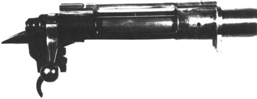
Figure 5-4 - Photograph of the steel bridge mount on the rifle action, which was used to solve the scope mount axial differential loading problem.
