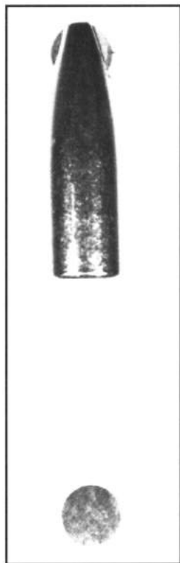
Figure 8-7 - Photograph of a 270 bullet with the magnet inserted in the 1/16 slot milled into the nose. A rare earth magnet is shown below the bullet.
