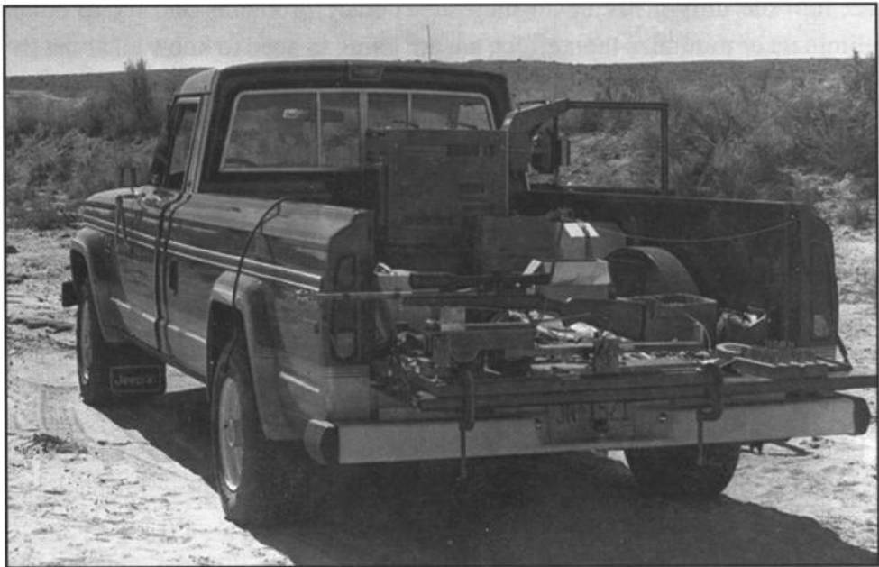
Figure 2-1 - Photograph of the field test setup showing the rifle mounted on a machine rest and the electronic instrumentation.
