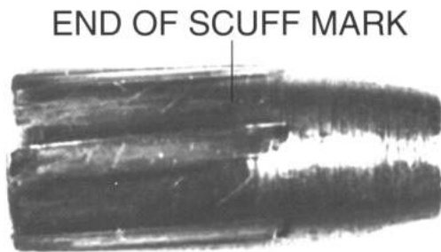
Figure 7-8 - Photograph of a recovered 90 grain 270 HP bullet showing triangular shaped scuff marks on the side wall of the bullet between the rifling marks, which can be measured to determine bullet cant.
