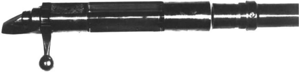
Figure 6-12 - Photograph of an action showing a disassembled barrel joint design that is immune to temperature and other barrel joint problems. This design is also depicted in Figure 6-11.
