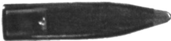
Figure 10-10 - Photograph of a 270 bullet with a light plastic cylinder swaged into the rear of the jacket behind the lead core. This moved the CG forward enough so that the bullet was stable in a 16 twist barrel. This jacket would normally result in a 150 grain bullet, but this bullet weighed 100 grains with the plastic insert.
