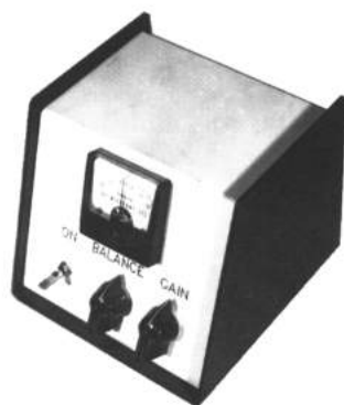
Figure 10-17 - Photograph of the indicator on the bench for the electronic wind gages. When the wind is from the right the meter needle moves to the right and just the opposite for a wind from the left. The goal is to fire when the needle is in the same place.
