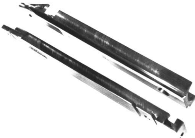
Figure 4-8 - Photograph of the Dado Slide recoil isolator device that proved to be less satisfactory than the Recoil Isolator using flexural beams.
