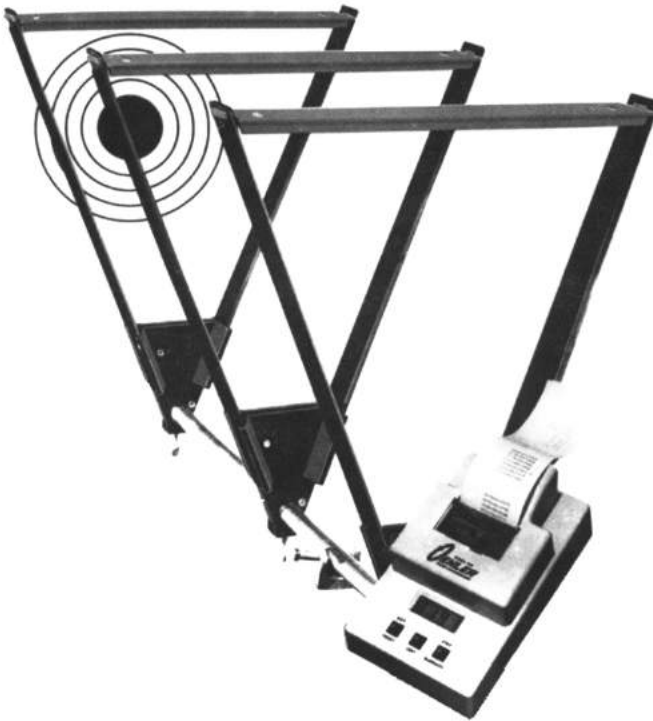
Figure 10-23 - Photograph of a modern state-of-the-art chronograph (Oehler 35P) with three optical gates. This chronograph uses electronic chip technology for computation and has a built in printer that records all the data. It measures velocity within 2-3 fps at 3000 fps. The optical gates are much more convenient than other types of triggers.
