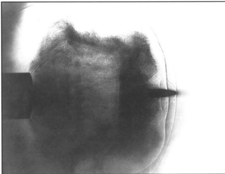
Figure 7-17 - Shadowgraph showing the bullet penetrating the main blast wave and starting to penetrate the precursor at 90 \mu sec. The main blast wave is overtaking the precursor. The bullet is out of any significant effect from the muzzle jet. There are tiny unburned powder particles trying to penetrate the blast wave above the bullet.
