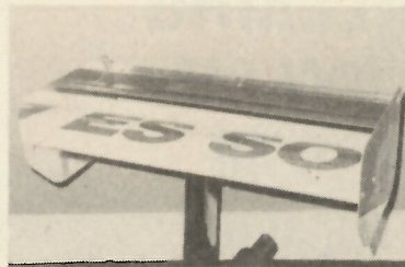
Argo JM14 FF2000 detail. Above: Lightweight centre-post wing carries Esso's message. Below, downwards: Narrow but functional cockpit; cleverly ducted engine cover and fully faired-in rear suspension for improved airflow.
