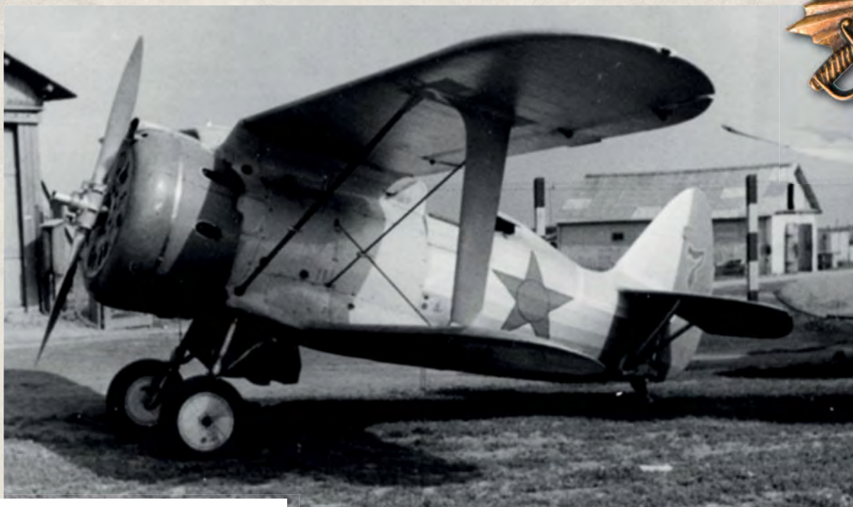
Left Tactical number '7', an agile I-153 powered by a 1,000hp M-62 radial.
