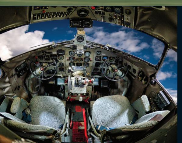
The cockpit of this C-47 has changed little since it left the factory. This interior is of a C-47 that flies out of Minot, North Dakota to this day. The only modern thing in the cockpit when it's being flown is a GPS unit they connect for flight. It's been to Oshkosh a number of times carrying the opening ceremony parachute team. (Photo by Jim Hazeltine)
