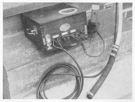
(Above) Components of the Burnand Timing Comparator comprise "hockey stick," starting Comparator equipment, automatic finishing device and main operating control.
