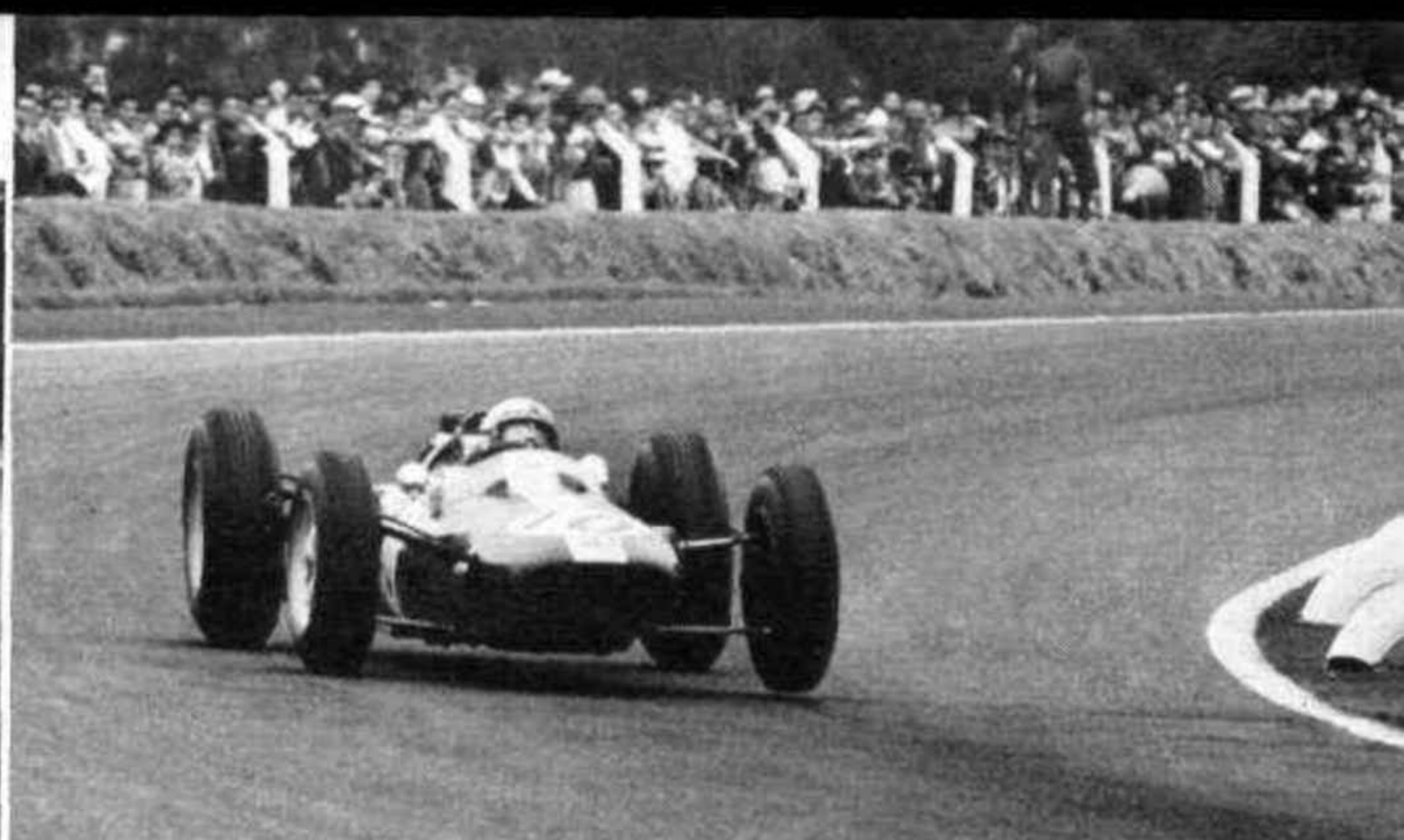
WHEEL LIFTING.—Rodriguez' (Lotus) inside front wheel lifting as the opposite rear suspension begins to break. The Mexican finally stopped when oil smoke from the distorted gearbox mounting brought him into the pits.
