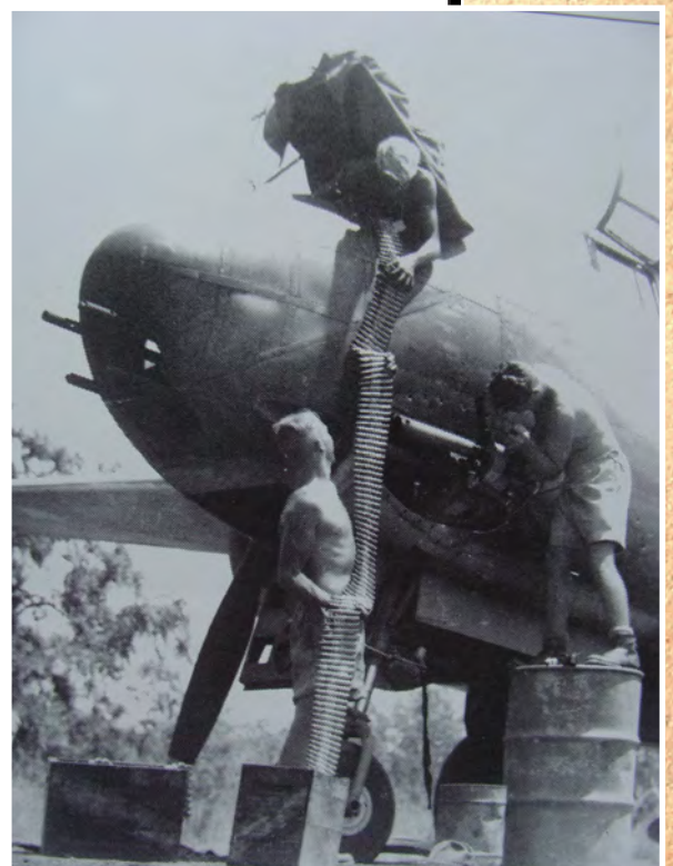
BELOW Ground crew replenishing ammunition for a 22 Squadron Boston's .5 inch machine-gun while another man works on its .303 inch guns at Ward's Strip.
