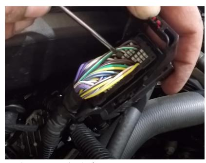
Plug the new pin from the Flex Fuel Harness into the slot for Pin 38.
