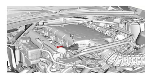
Attach Flex Fuel Harness to the GM Flex Fuel Sensor. Route the harness wiring along the left side of the engine cover until you reach the EVAP Sensor plug in.
