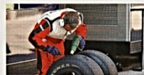
2:39 PM 21 LAPS GONE Bridgestone 'scrape' the used tyres to analyse wear rates
