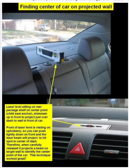
Important note: Specifically in the Jetta, make sure you adjust the high beams first using the L2/H2 adjustment. This adjustment moves both the high and low beams together. Next, after you have the high beams correct, then you can adjust the low beams both up and down (L3) and left and right (L1) to meet the spec.
