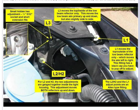
So, what follows is the procedure I used to adjust my headlights. This technique basically lowers your high-beam aiming down to a good position while returning your low-beam aim to the same point they are now.
