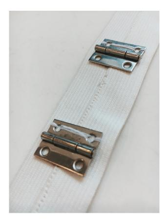
Stitching **three wearable parts** - the neck, waist and hip, to ensure that the structure **follows the spine as closely as possible** when worn.
