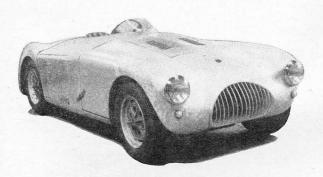
Dimensions:-Wheel base 7' 6". Track 4' 2". Overall width 4' 10". Height to scuttle 3' 2". Overall length 11' 2". Ground clearance 5".
