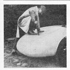
FOOT DOWN: R. G. Shattock demonstrates the flexibility of the R.G.S. fibreglass body . . .
