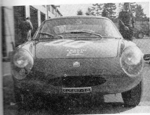
SMOOTH LINES are those of the 1964 2-litre Abarth G.T. car, which is apparently built on a Simca platform chassis. The car uses a six-speed gearbox and the all-Abarth engine, which develops 180 b.h.p., is equipped with horizontal Webers. If homologated, the 2-litre Abarth will be out for Porsche blood.
