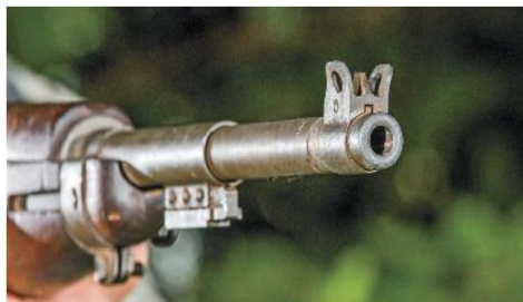
The carbine features a protected post front sight which is non-adjustable but provides a good sight picture.
