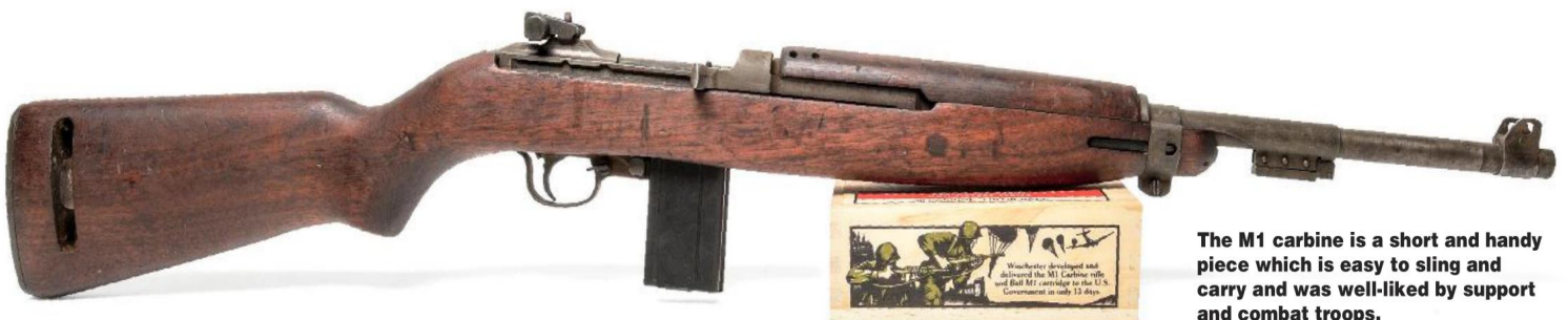
The M1 carbine was developed to be significantly lighter and handier than an M1 Garand rifle or the Thompson submachine gun while being more effective than the M1911A1 pistol.
