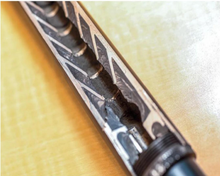
If you don't clean your rimfire or pistol suppressor, it will get gunked up like this one. 3-Ring Silencers can all be taken apart for cleaning.
