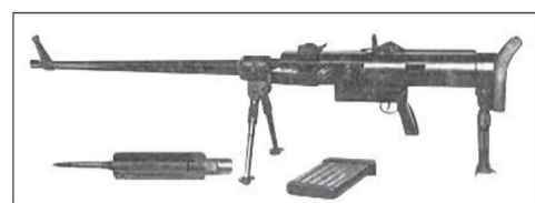
Photograph of an Oerlikon SSG36 with the bolt and magazine in the foreground.
