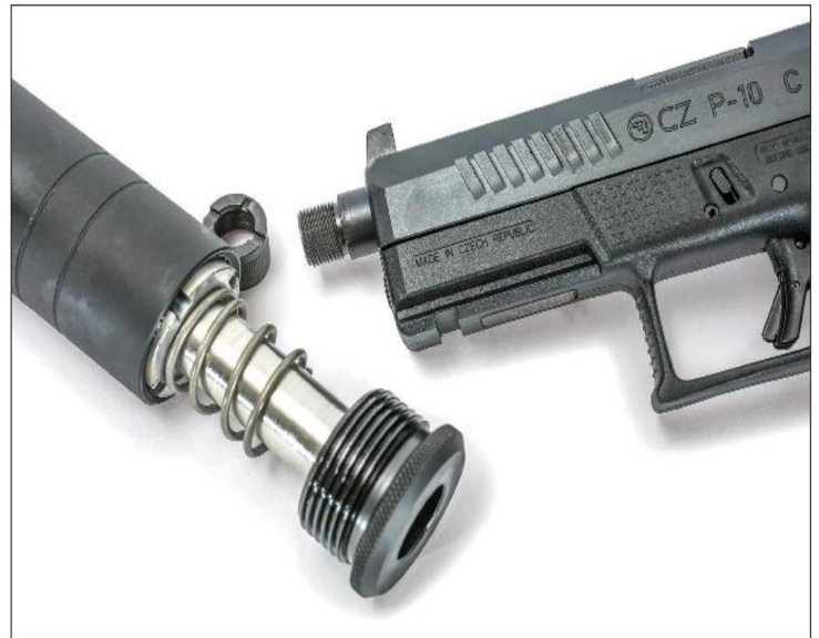
The thread protector off of the pistol barrel, and the rear cap of the 3-Ring silencer unscrewed, to show the booster and spring.
