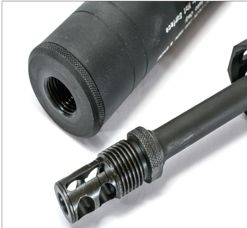
The 762 muzzle brake in place, ready for the silencer mounting.
