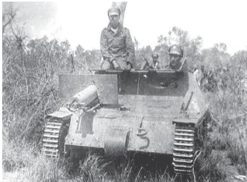
A 7.65 Vickers mounted on a Bolivian Carden-Loyd Tankette.
