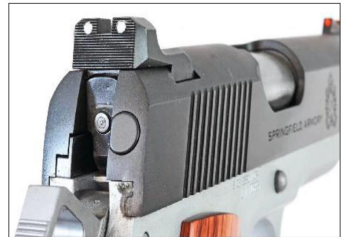
The rear sight is serrated and beefy, with white dots to either side of the notch. The Ronin Operator has a traditional 1911 tensioned extractor.
