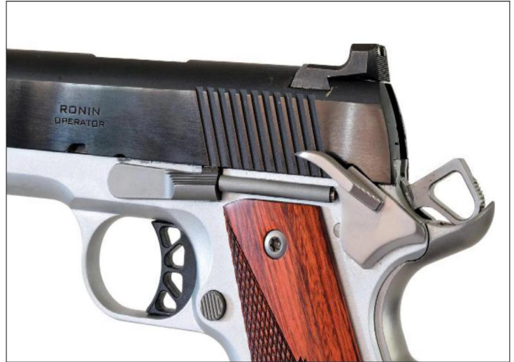
The Tactical Rack rear sight features a vertical face on the front so you can rack the slide one-handed on a hard surface. The slide serrations have flat bottoms and are a bit more aggressive under the finger than the traditional angled serrations.
