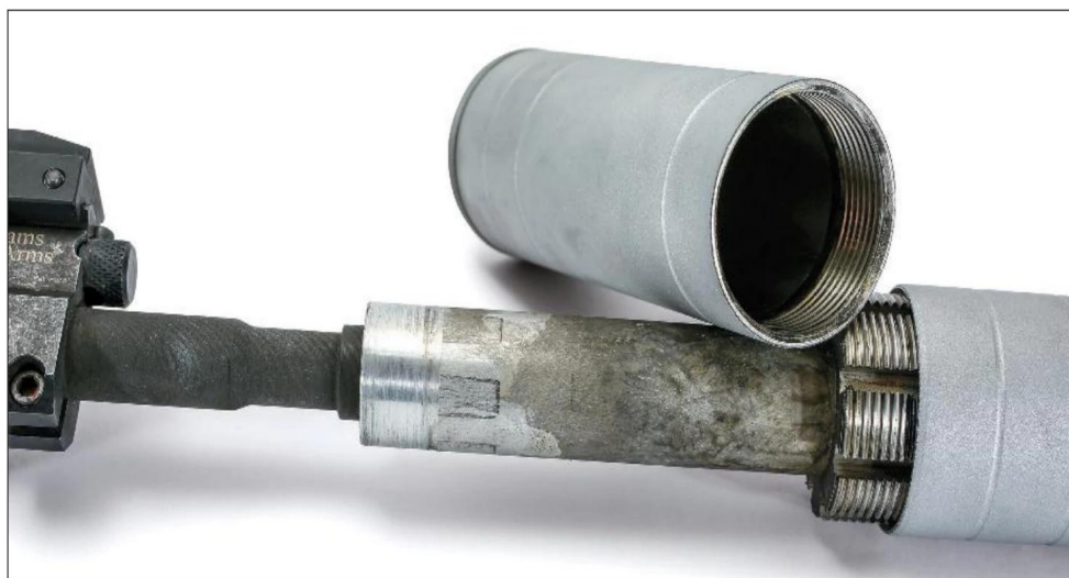
Here is the rear half of the OTB silencer taken apart, to show the barrel overhang, and the area you can clean, when you need to.
