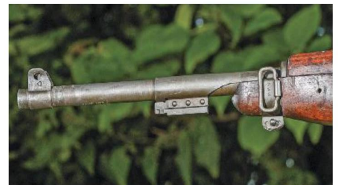
Later production guns were fitted with a bayonet lug based on after-action reports from combat troops.
