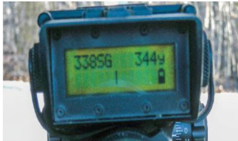
Ballistic calculators such as the BORS (Barrett Optical Ranging System) calculate much of the information a CT sniper needs for a shot.
