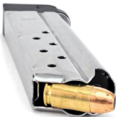
Modern 9mm 1911 magazines feature spacers to keep the shorter rounds from moving inside the .45 ACP-length magazine bodies, and departing the feed lips at the same point every shot.
