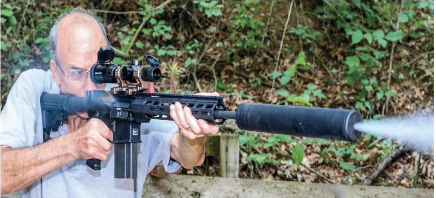
A 7.62 rifle produces a lot more gas, because it is burning more powder and pushing a heavier bullet. So, you need a bigger silencer than a 5.56 carbine needs. Even so, a silencer built to handle a 300 RUM is bigger than a 7.62 NATO rifle needs. Quiet, though.
