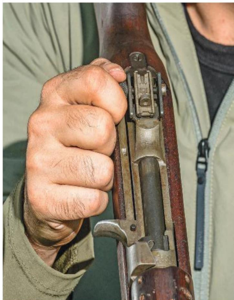
While a simple dual-aperture flip-sight was initially issued later a more refined fully adjustable rear sight was fitted.
