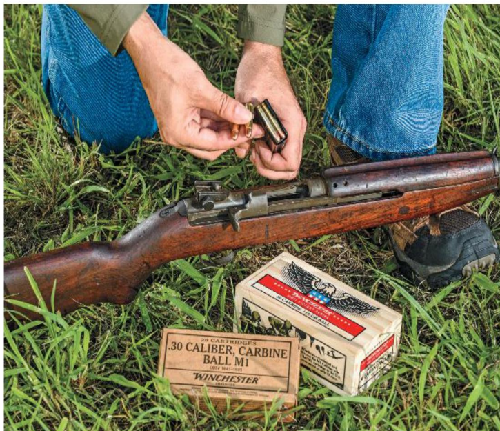
15-round dual-column dual-feed magazines were issued with the carbine, later a 30-round magazine was issued with the introduction of the selective-fire M2 carbine.
