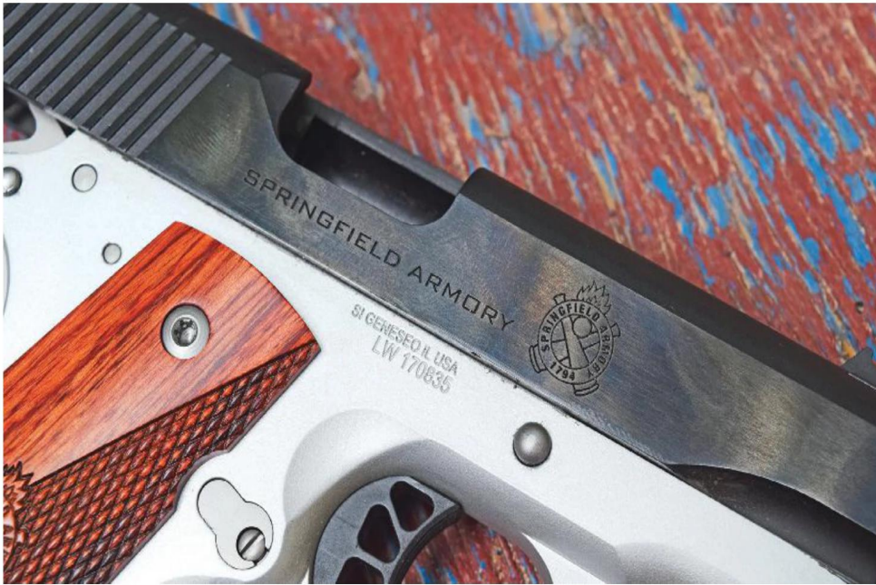
The flats of the slide have been polished, and in combination with the bluing provide a very classy look. All the logos, names, and numbers on the pistol are laser etched.
