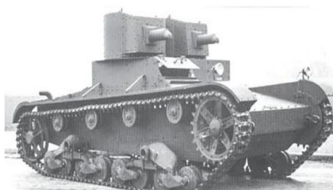
A Bolivian Vickers six-ton Type A tank with a 7.65 Vickers machine gun in each turret.
