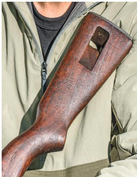
The buttstock features a sling slot which also holds an oiler. The sling position allows the carbine to lay flat against the back for comfortable carry.
