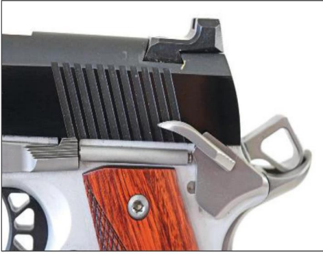
The Tactical Rack rear sight features a vertical face on the front so you can rack the slide one-handed on a hard surface. The slide serrations have flat bottoms and are a bit more aggressive under the finger than the traditional angled serrations.
