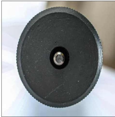
An alignment check, on the 200 and 175 556 silencers, both produced perfect alignment.
