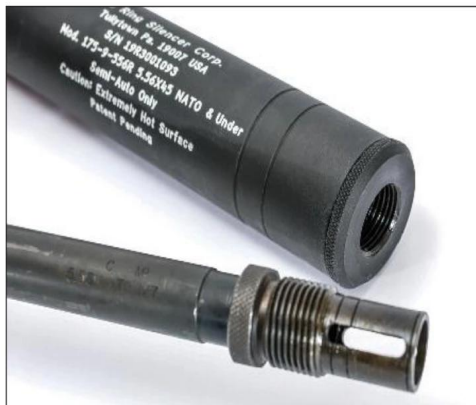
Here is the 175-9 rifle silencer, and the flash hider that comes with it. The silencer threads onto the flash hider with the threads you see, so make sure your flash hider is locked down with Rocksett.
