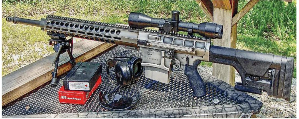
DRD Tactical's Kivaari is a .338 LM sniping rifle that may be taken down and carried in a backpack. It has received interest from various CT units.
