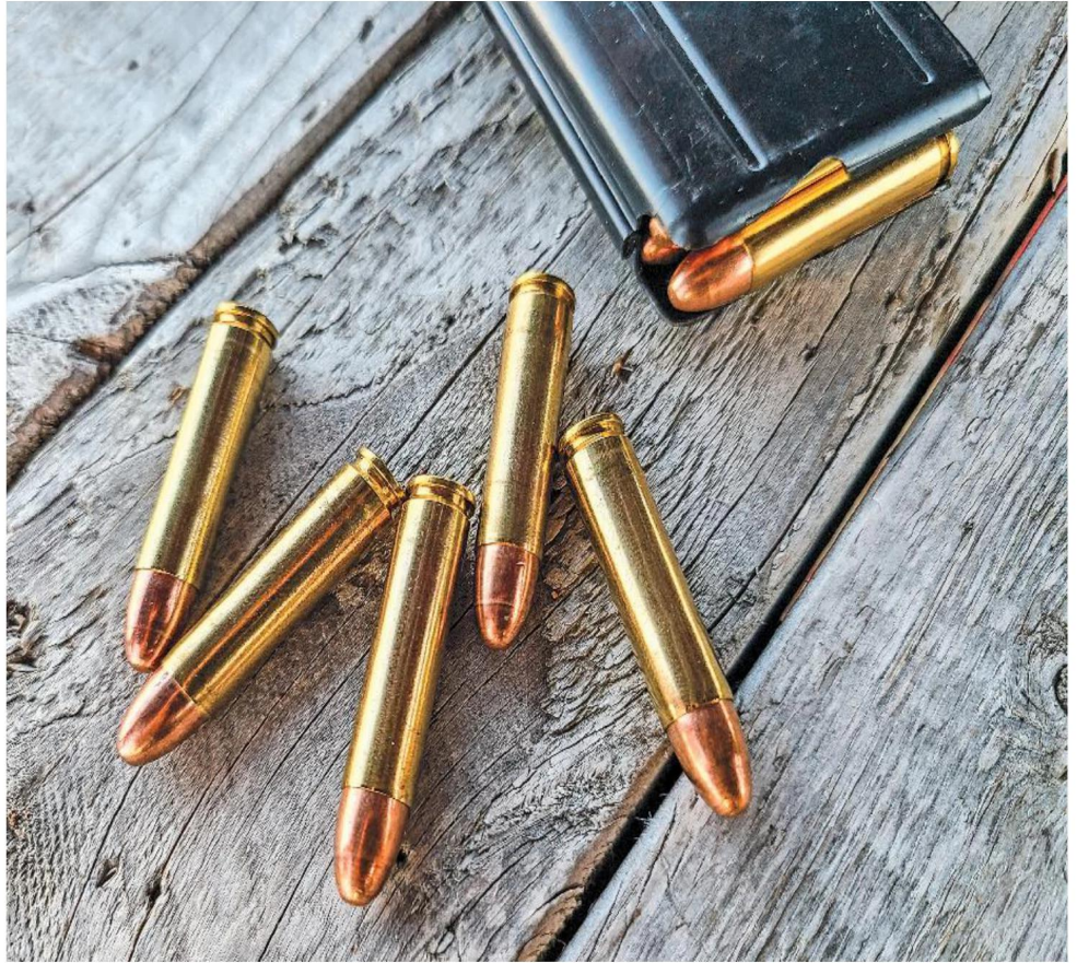
Unlike the .30-'06 M1 rifle, the M1 carbine chambers a lower power .30-caliber cartridge developed expressly for it and based upon the old .32 SL. It is loaded with a 110-grain FMJ at about 1,990 fps.
