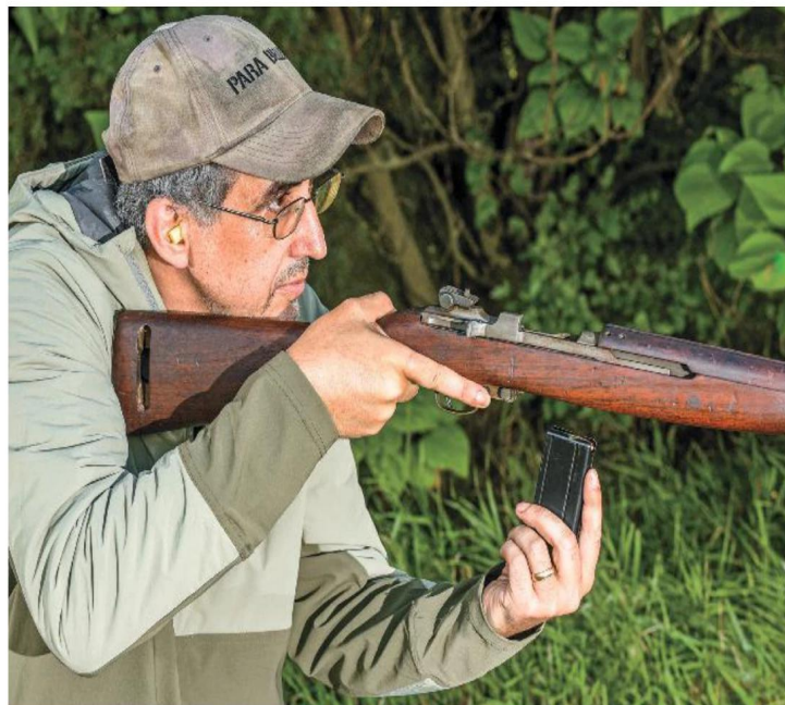
Magazine insert with a simple upward push and can be removed by depressing the magazine release button.
