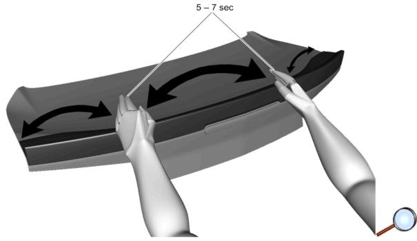
17. Apply pressure to entire spoiler surface. Ensure that all clips are engaged.
