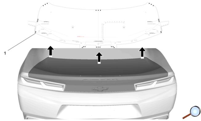
8. Fold the template (1) upwards and secure for later use. Use tape to keep template clear of work area for drilling.
