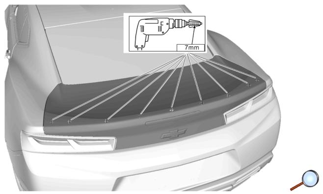
9. Drill a 7mm hole at all the punched center for each hole.
