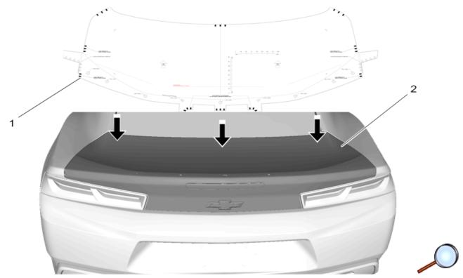
4. Position template (1) on rear compartment lid (2). Follow the instruction on the template for layout procedure.
