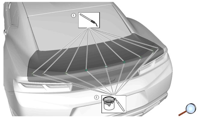
15. De-burr drilled holes and apply P/N 12346225 to all holes.
