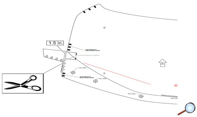
21. Cut on the inner dotted-line at the shown location so the section of template is flush with the deck-lid to ensure the 6mm (min.) gap. Cut approx.1.5 in. to remain attached to the template.
