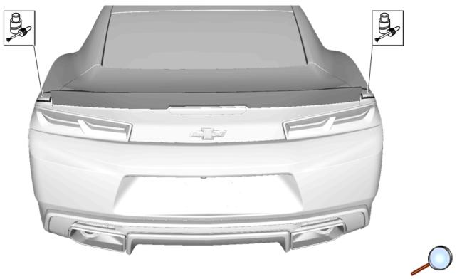
25. The bonding surface on the quarter panel surface to be primed with 3 applications in intervals of 5 minutes between each application. Remove Primer Template after last application.
