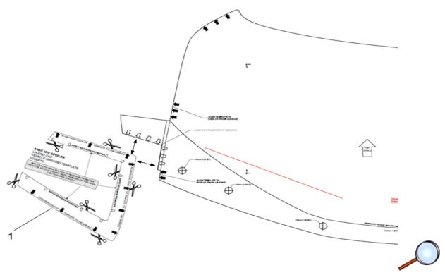
24. The Primer template (1) should be positioned as shown above.
