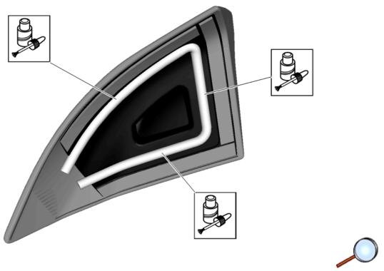
23. The bonding surface on the inner surface of the end caps to be primed with 3 applications in interval of 5 minutes between each application with Primer.
