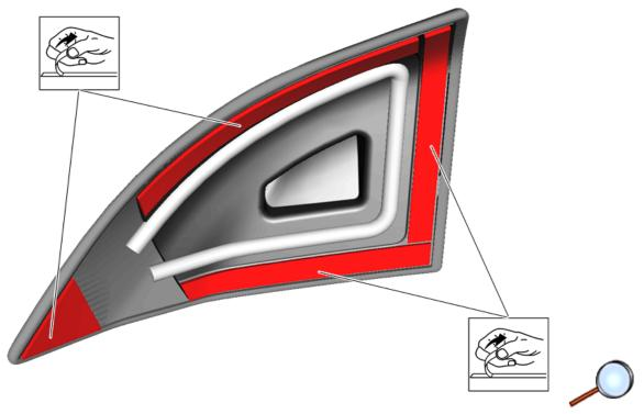
27. Start the pull the tape tabs from end caps ensuring not to smudge the adhesive bead.
