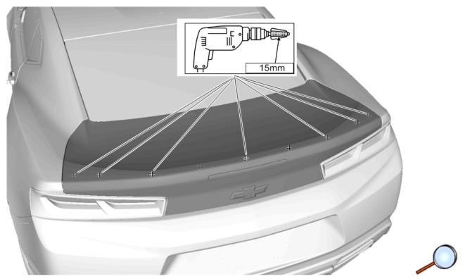
11. Drill 15mm holes according to locations specified.
