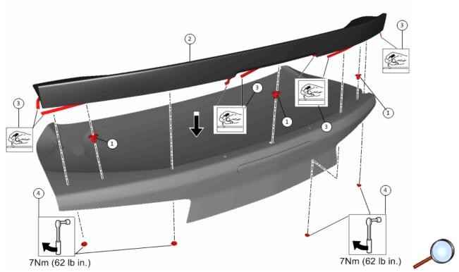
16. Insert the stud retainer into the center and the second out-board hole on each side. Start the tape and set the spoiler to rear compartment lid. Ensure the stude engage into the retainers. Pull the tape tabs. Install the nuts and tighten to 8 N.m (71 lb in).
