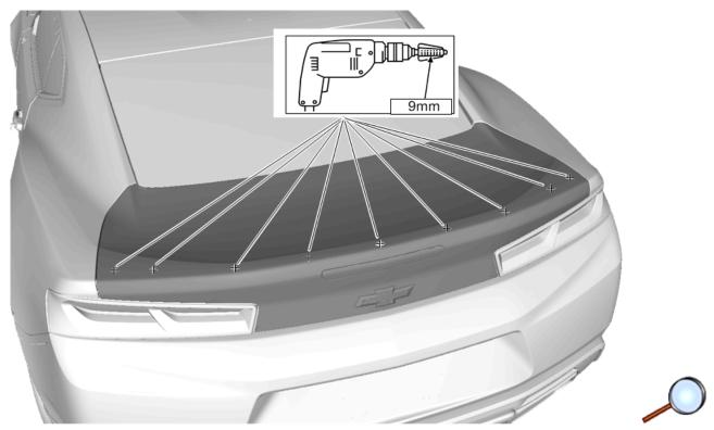
10. Drill 9mm holes according to locations specified.
