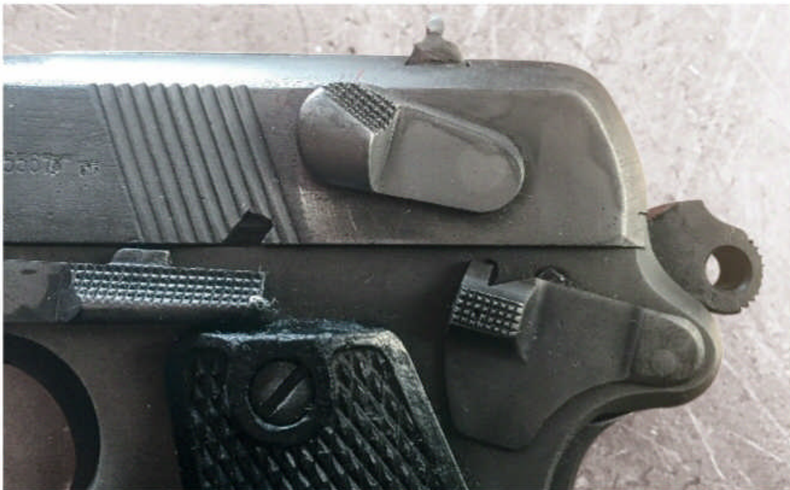
▲ The Radom Vis-35 featured a decocking lever, which was unusual for a military pistol of that era. Final versions dispensed with the takedown latch (rearmost control on this sample).
