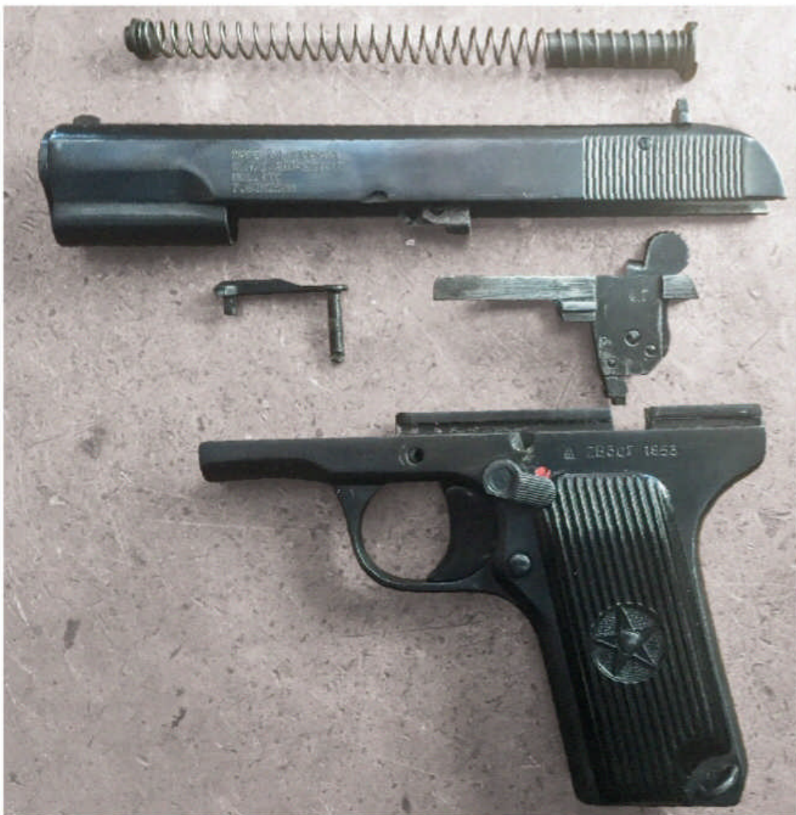
▲ The TT-33 has a modular, removable hammer/sear fire-control unit. This sample includes a manual safety mandated by import rules.
