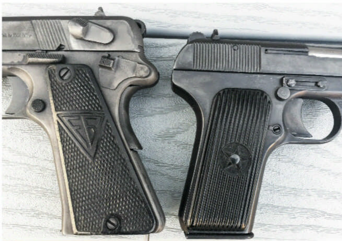
▲ The grip of the Tokarev TT-33 (r.) may seem less pointable than that of the more hand-filling Radom Vis-35, but the actual grip angles are within a half-degree of one another.
