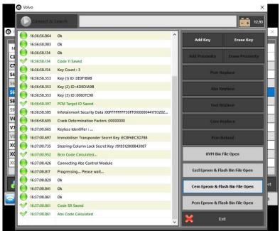
After the operations in Cem and ABS units are finished, it is time to prepare pcm bin.file...
