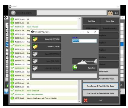
After uploading the files belonging to PCM, the last thing we will do is to press the Syncrho button. The synchronized bin.file will be saved to the location you specify...
