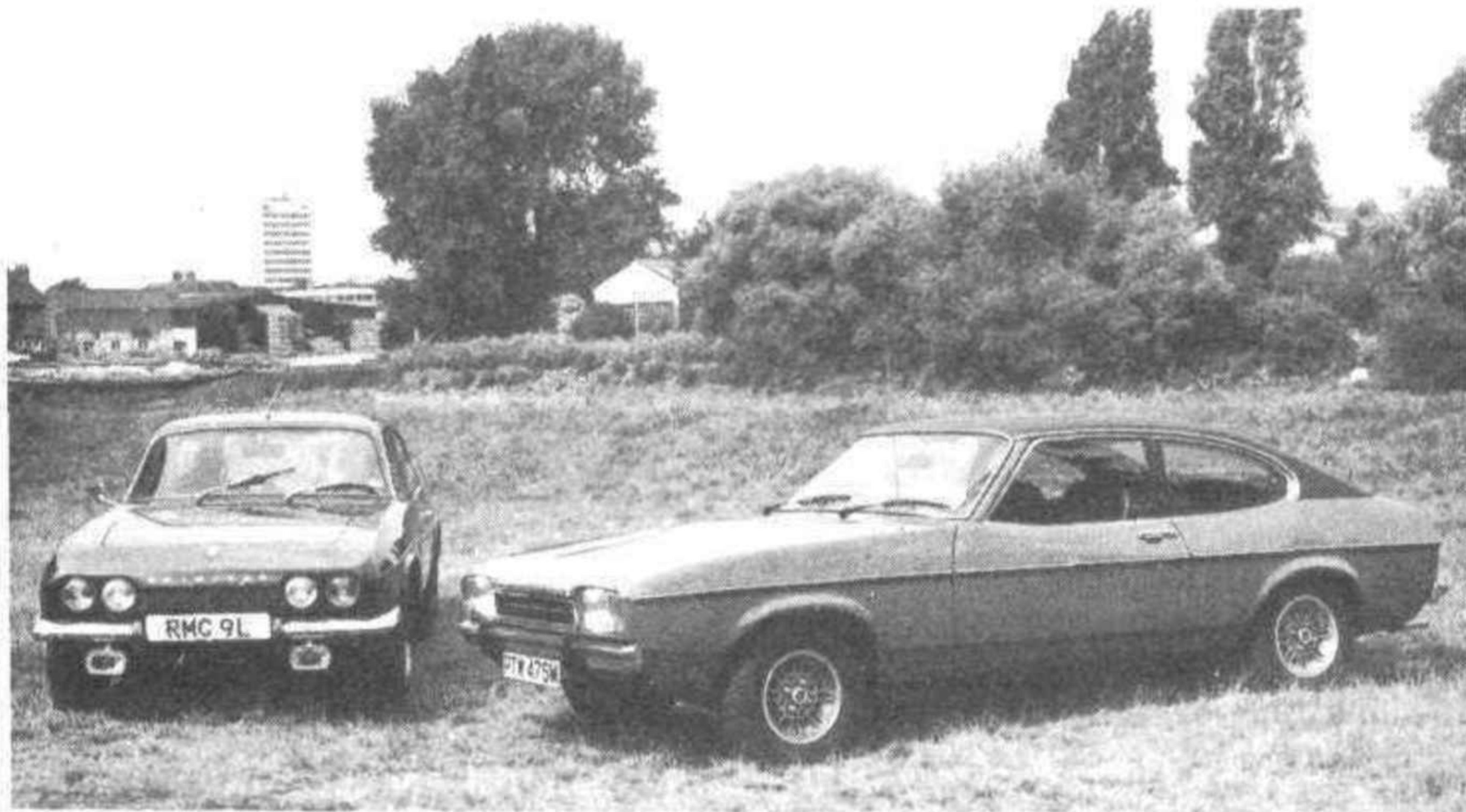
Two sporting estate cars with the same Ford 3-litre V6 engines, a choice of steel or glass-fibre construction and very different characters.
