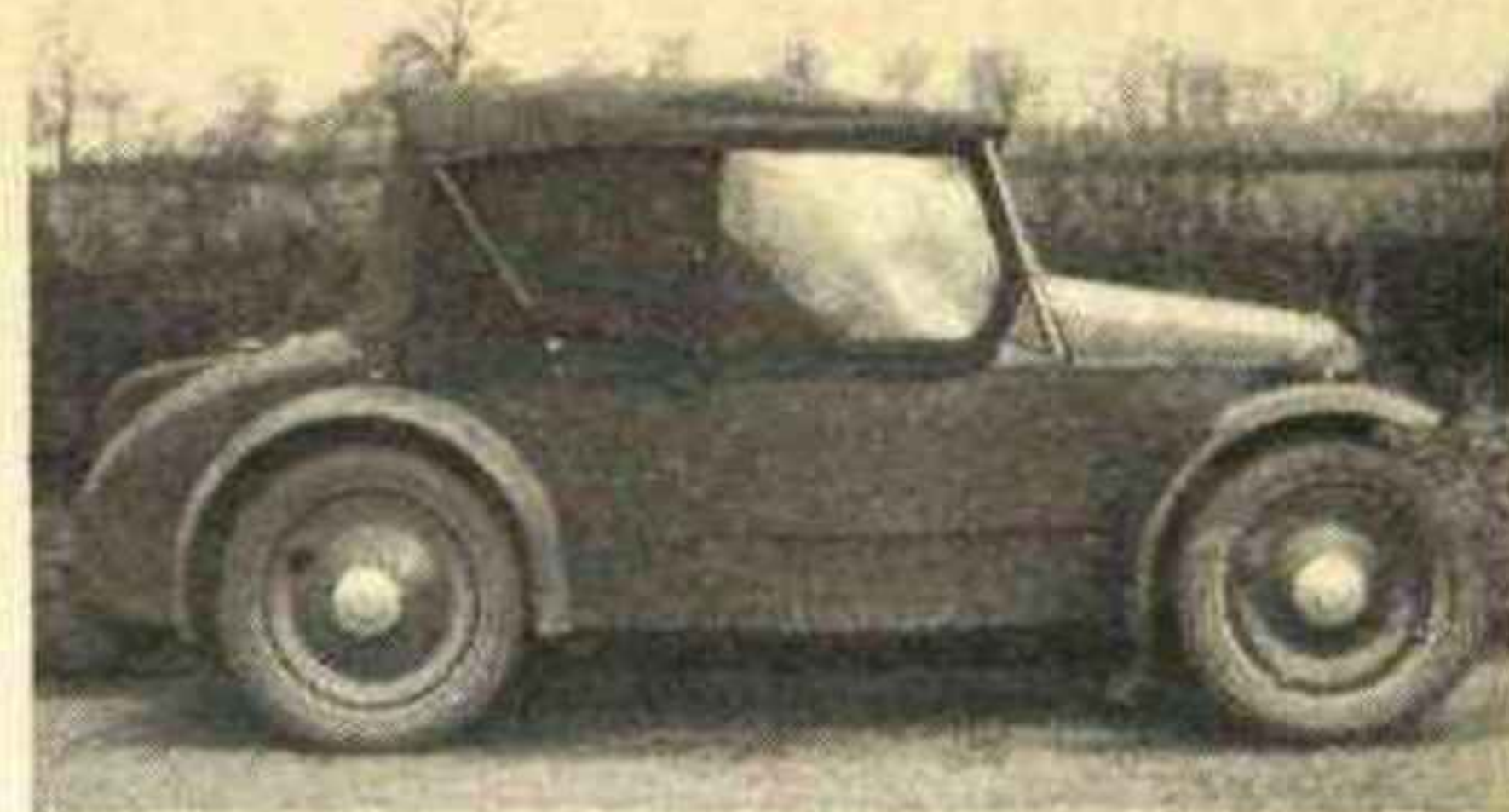
Side view of the rear-engined, air-cooled 840 c.c. Rover Scarab. Note the all-weather equipment!
