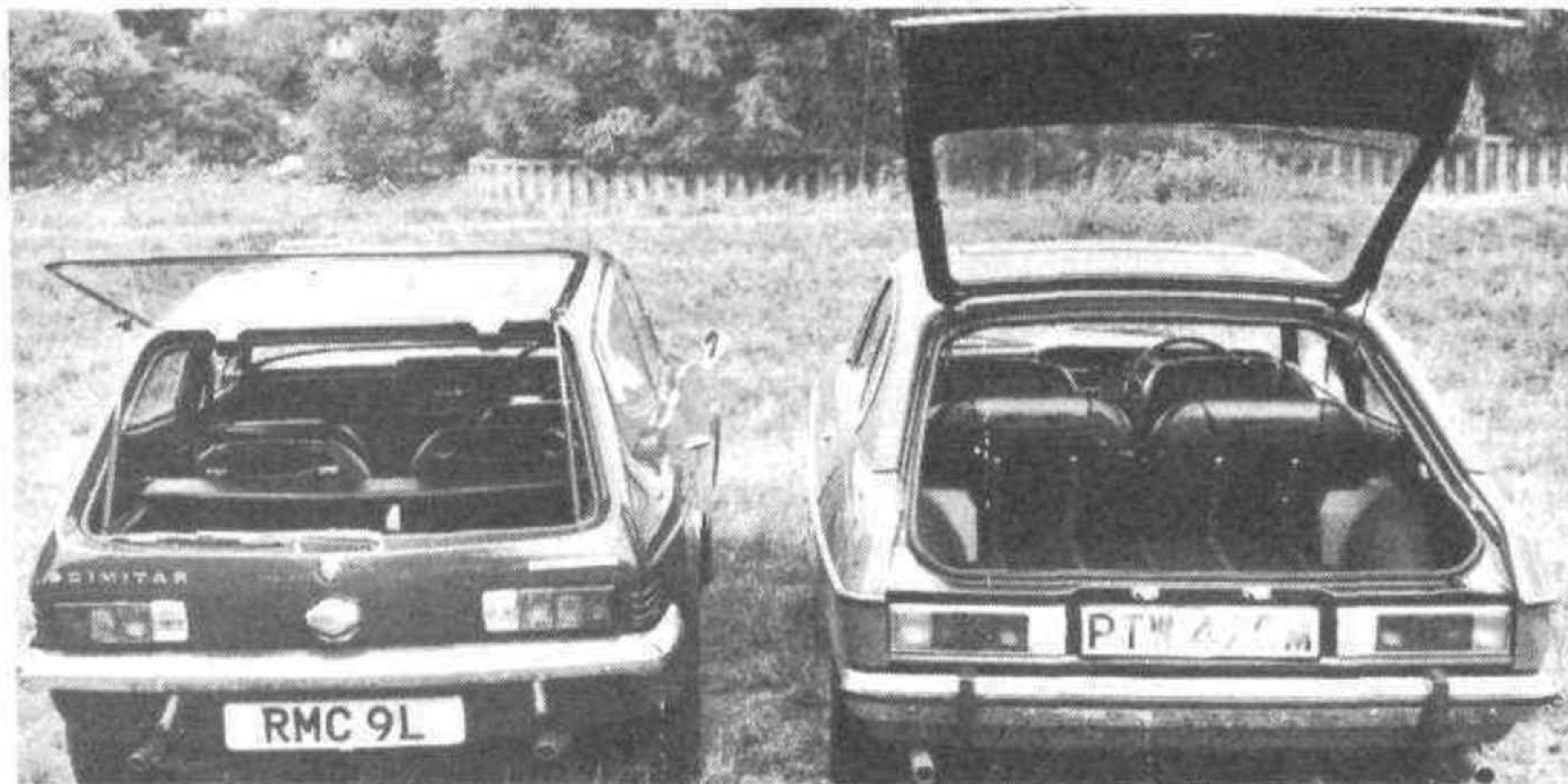
The Capri's much larger tailgate is convenient, but the sloping roof and protruding wheel arches make the bay a less convenient size than the Scimitar's.
