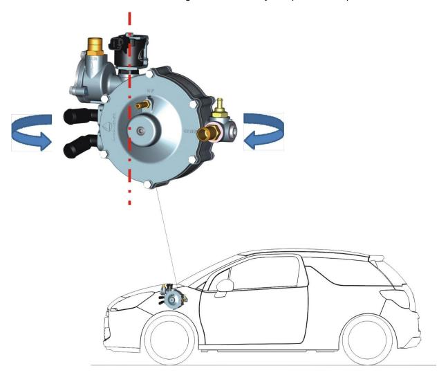
As shown in the figure, the regulator can be rotated on the axis of the solenoid valve, but it must always be facing upwards.
