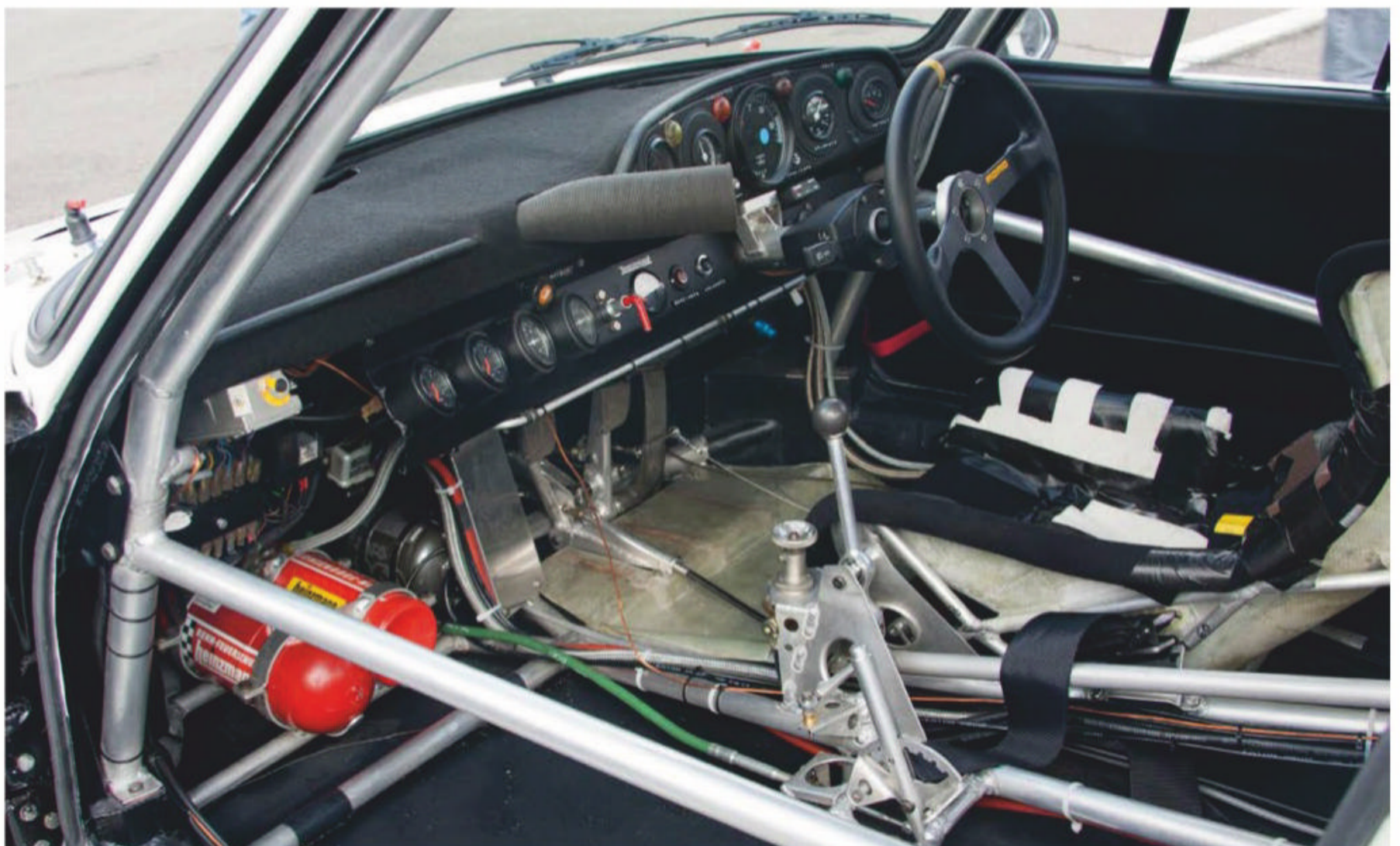
Because of a regulation change Porsche was allowed to raise the floor to the level of the sills. The shape of the cabin had to remain the same as the road going 911
