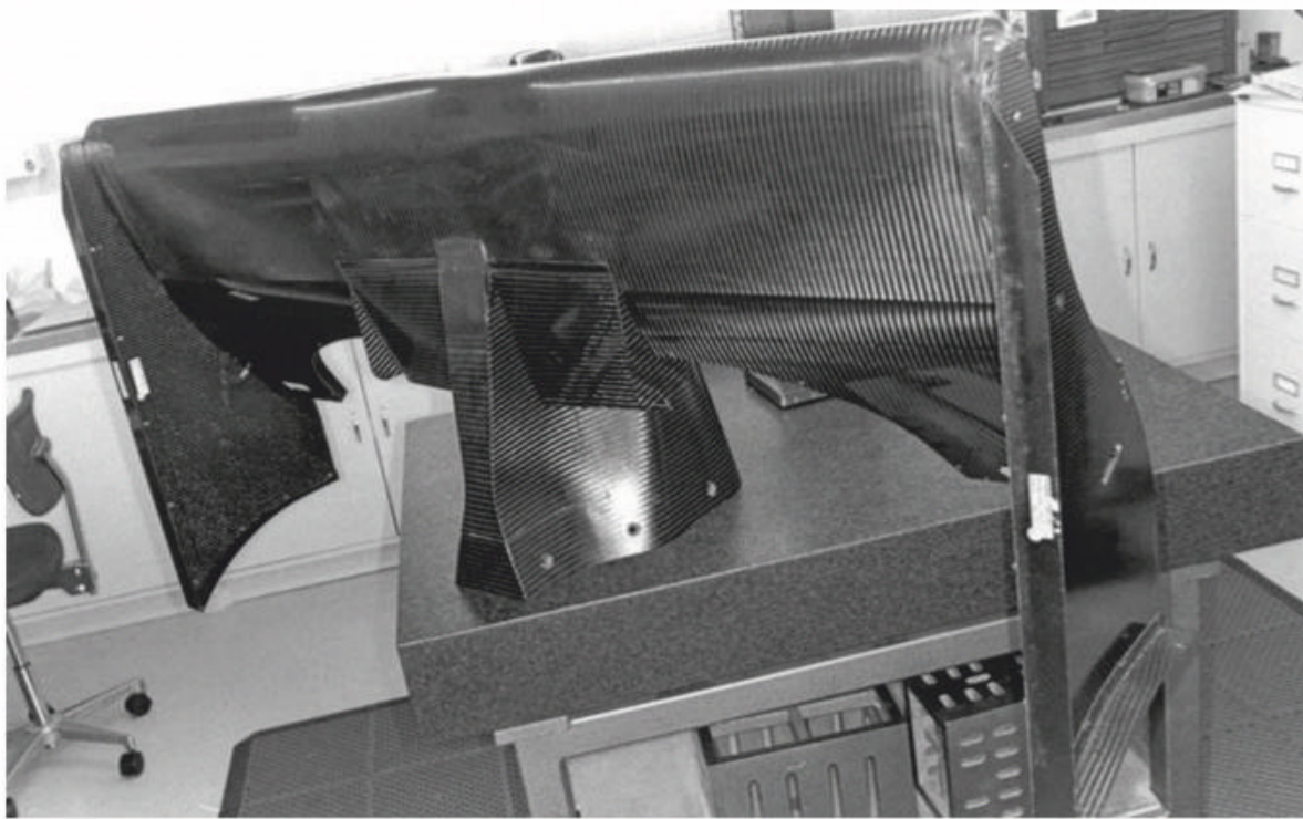
A view of the underside of the road course nose and wing assembly reveals the cutaway and the central keel
