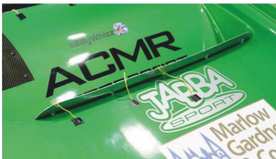
The radiator exit duct, which is situated in the front clam shell, has a prominent Gurney
