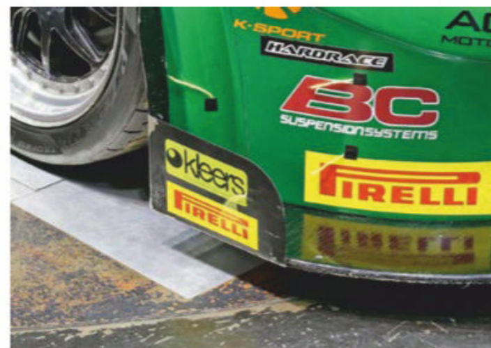
These simple splitter end fences proved to be potent devices
