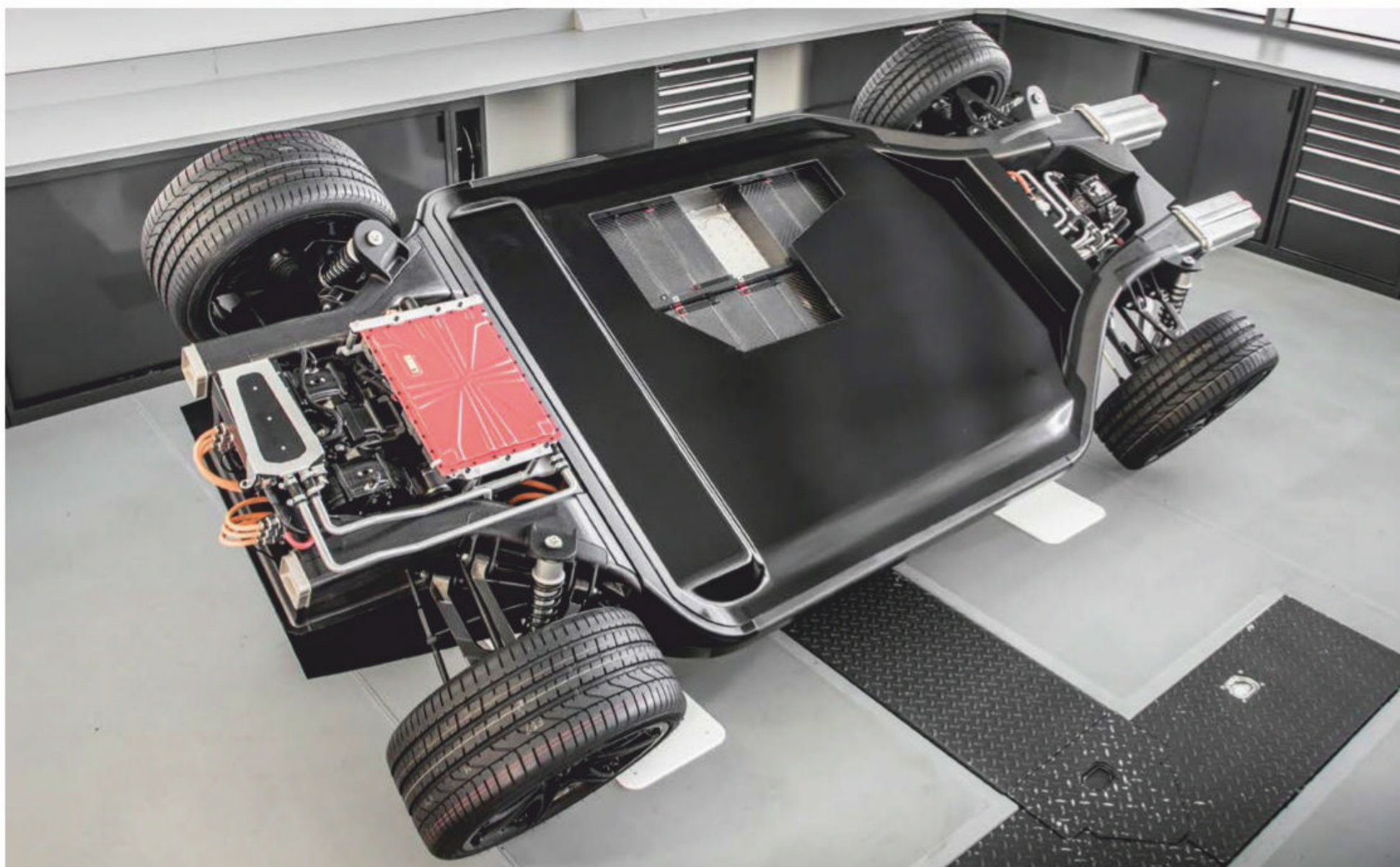
Both the 223 and the Racetrak composite technologies have been used to great effect in the Williams Advanced Engineering-developed FW-EVX electric vehicle platform concept
