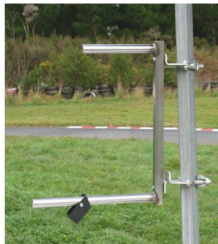
The box is easily slotted into bespoke low-cost tubular brackets
