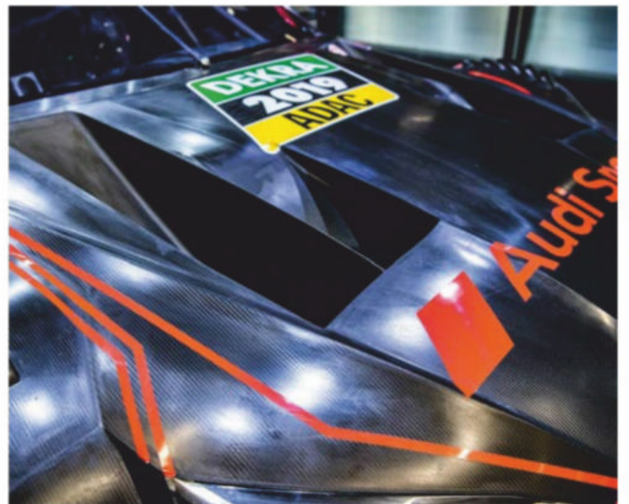
Provision for extra cooling is most evident on the bonnet. This is Audi's approach
