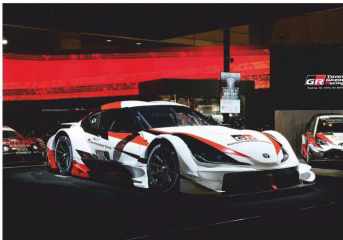
The new Toyota Supra is a small car so its dimensions have had to be stretched for it to fit the GT500 technical template
