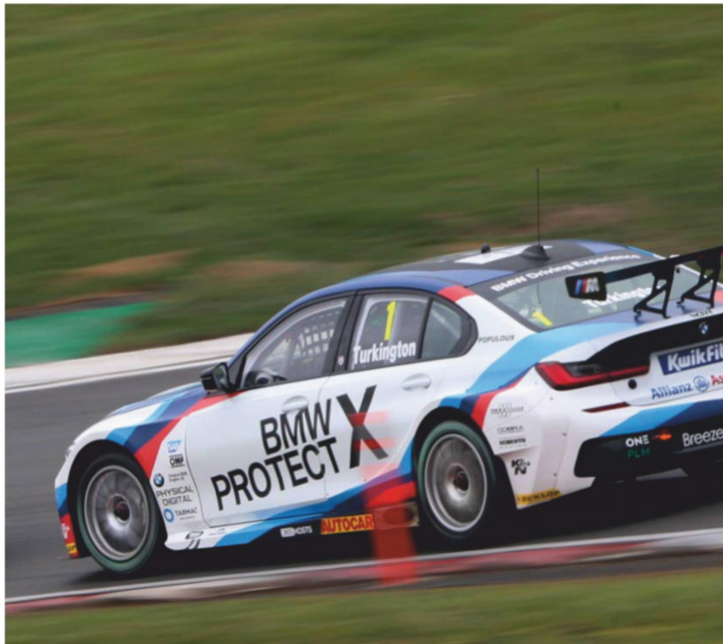
WSR has made the most of the larger cabin and has moved the driver towards the rear to improve the car's weight distribution
