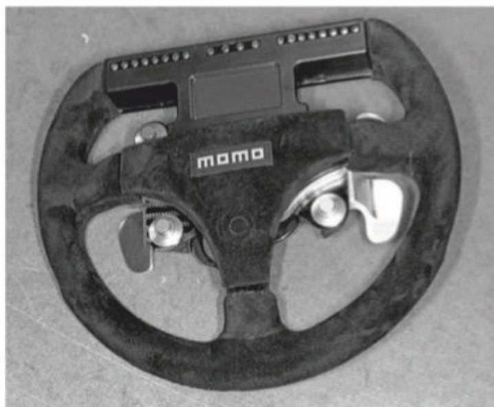
The wheel includes paddles for hydraulic corner weight jackers
