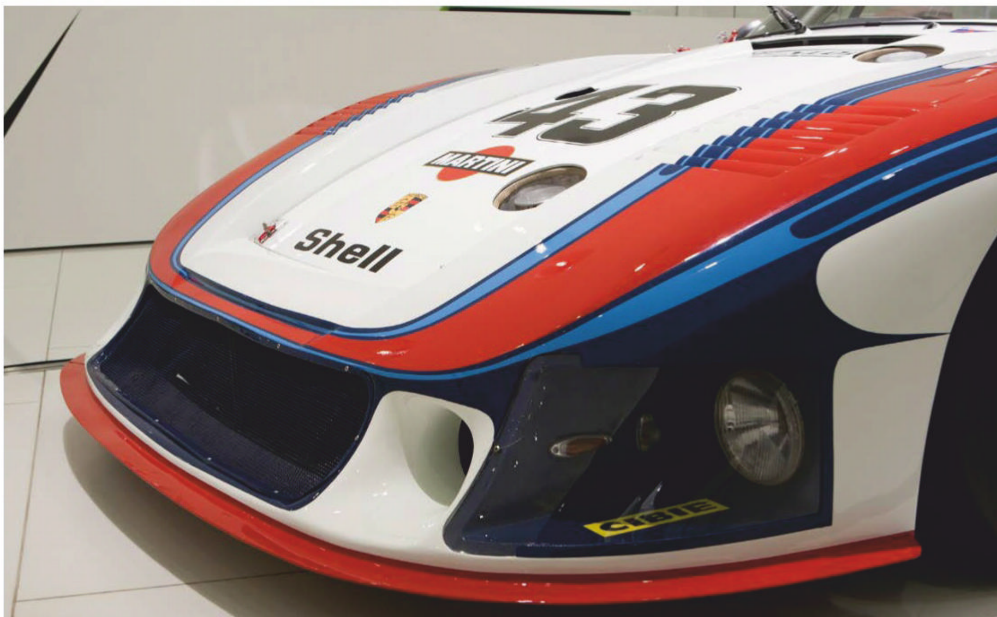
The Porsche 935/78 is justly famous for its slippery shape. The relatively long, wide and low nose was designed to reduce drag and to force the air over the body to the rear wing
