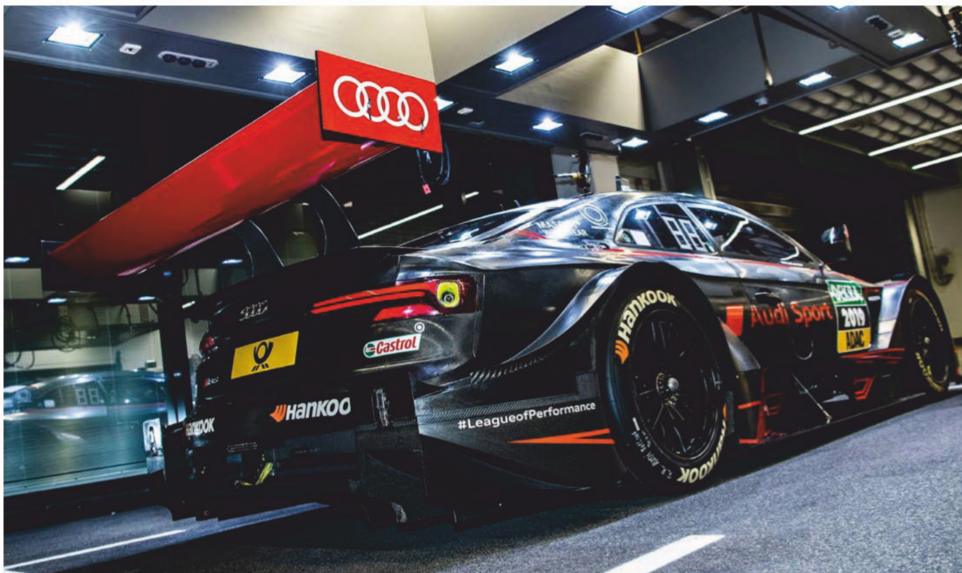
For this season the DTM cars are running with a shallower rear diffuser but the big aero talking point at the back of the car is the decision to run with DRS. There is also a new floor
