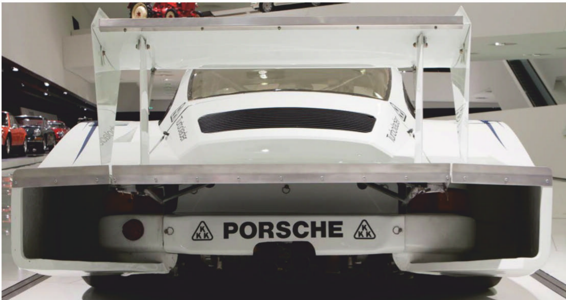
The rear wing had to be narrowed so that it was not visible from the front of the car, and it was then raised so that it would remain effective. From this angle there's very little 911 left
