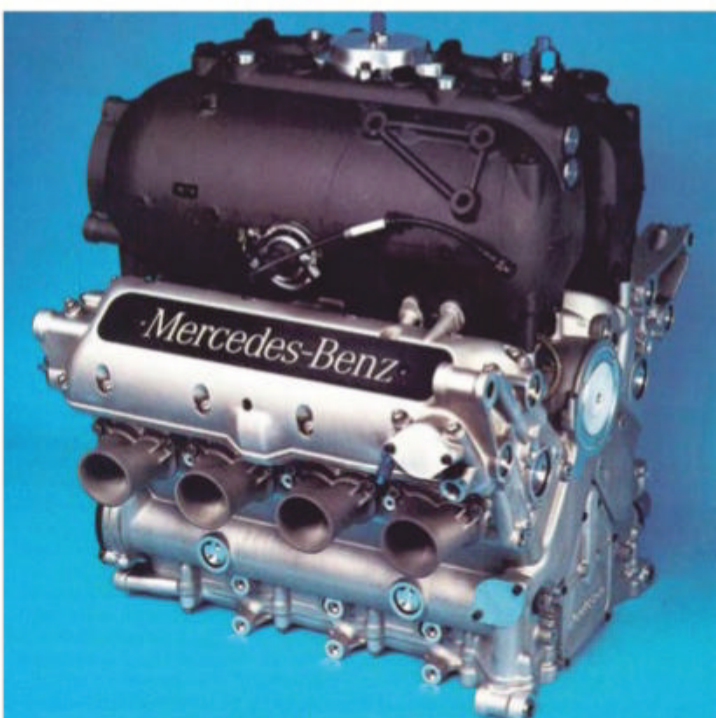
The Formula 1-inspired Ilmor engine that powered the PC27 was shorter, narrower and lower than the unit that was in the PC26
