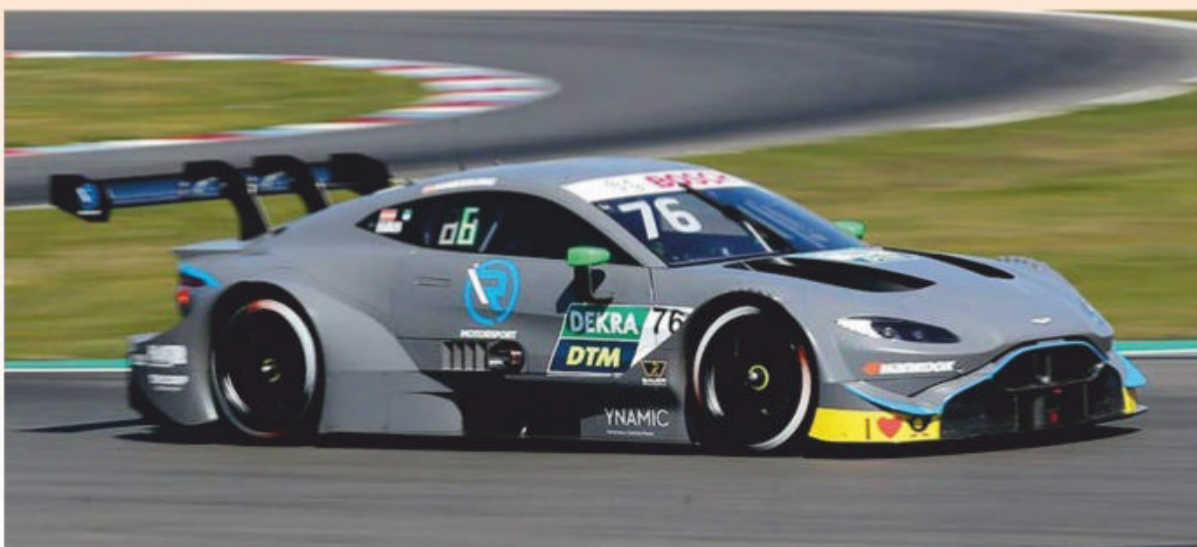
The Aston Martin has had to be stretched and also squashed down a bit to fit the DTM’s dimensional template
