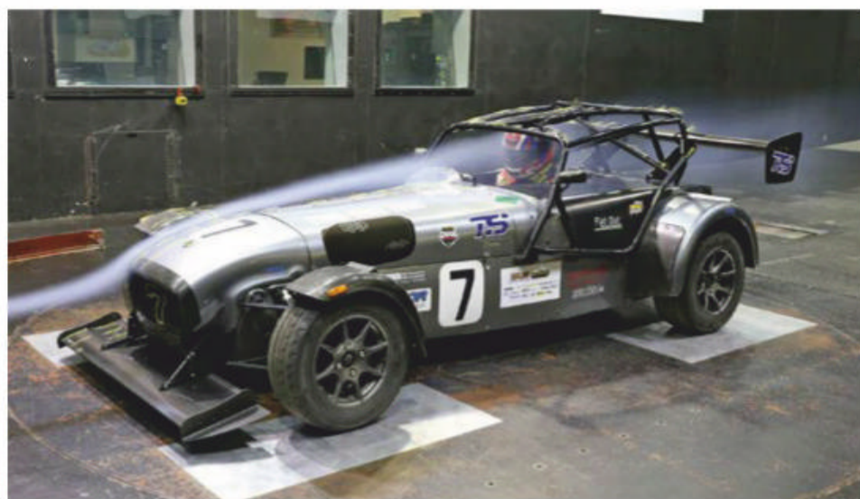
The Caterham had modest downforce figures, despite a recently fitted wing package
