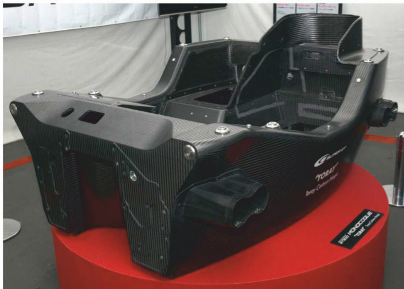
The 2019 GT500 monocoque. Revisions will come in 2020 but it will remain dimensionally identical to the DTM version
