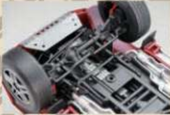
转向/避震/合金车架 Steerable Front Wheels / Active Suspensions / Diecast Body
