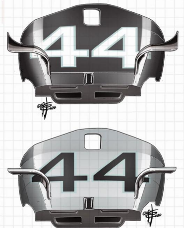
REPROFILED FINS ON TOP OF THE CHASSIS BULKHEAD
