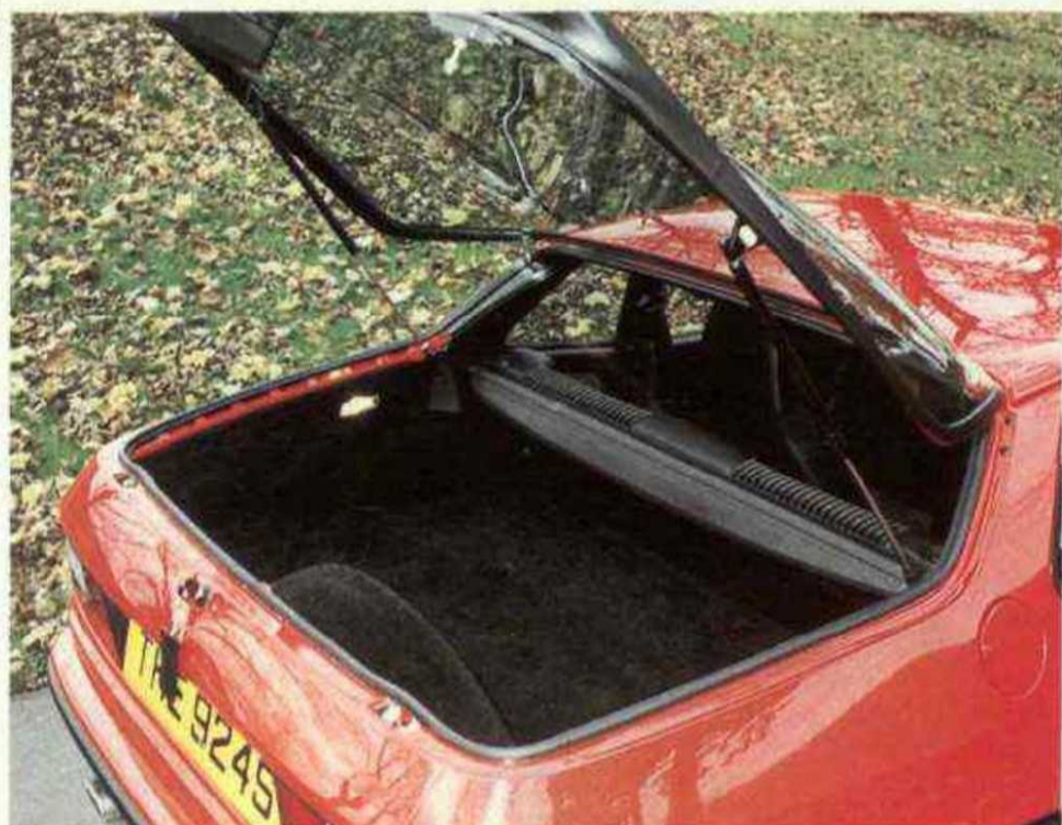
ALL-GLASS HATCH lifts easily to reveal shallow luggage platform with full-sized spare tyre. A neat roller-blind fixed to the backs of the folding seats conceals valuables. Window stays fairly clean but there is some distortion when looking through the curved sections.
