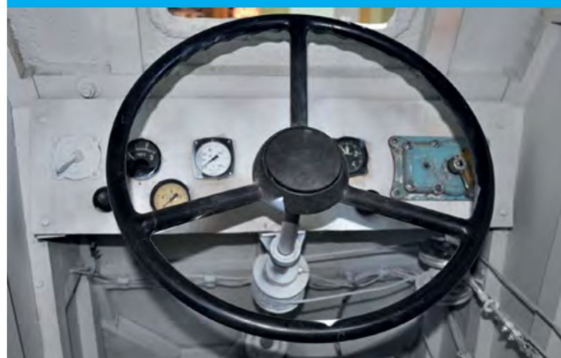
The NKL-26 driver-mechanic controlled the vehicle by means of a conventional steering wheel linked to the front skis
