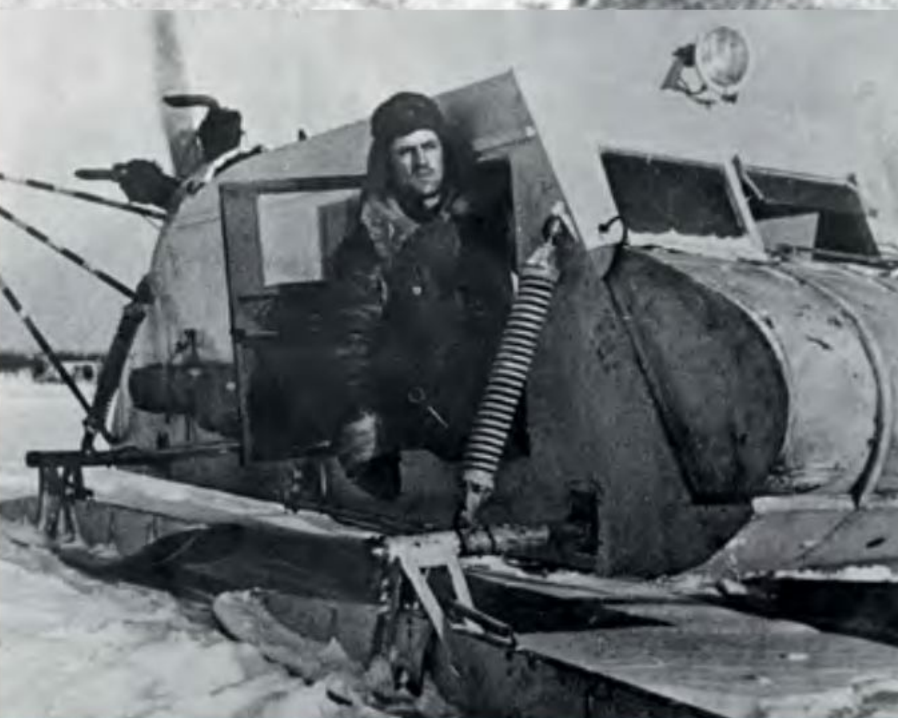
The commander of an NKL-16 M-1941 transport aerosan leaning out of his aerosan, near Staraya Russa. The strapped-on fuel tank is the primary distinguishing feature of the NKL-16 M-1941. Note also the red and white warning marking on the propeller guard and the spare propeller wrapped in canvas and strapped to the vehicle side. STEVE ZALOGA
