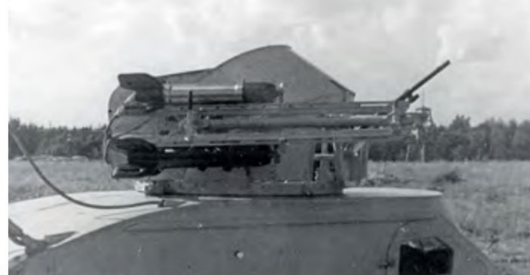
An NKL-26 M-1942 fitted with the 82mm RS-82 rocket launcher tourelle under evaluation at Kubinka in July-August 1942. The RS-82 aircraft rocket was the predecessor to the BM-8 'Katyusha' rocket launcher system. TSAMO
