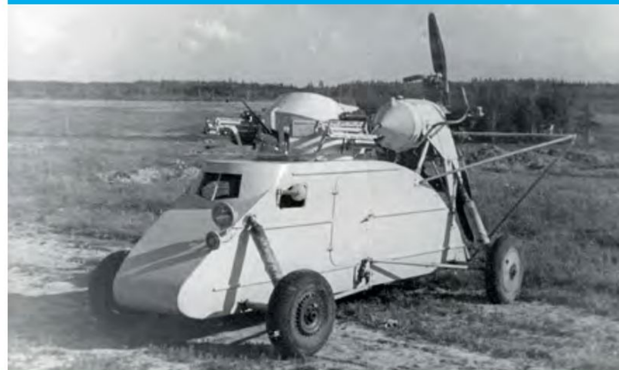
One prototype NKL-26 M-1942 was fitted with a tourelle mounted RS-82 rocket launcher system. The system proved to have had limited firing accuracy with the simple circle aiming sights provided on the prototype. It was also highly dangerous for the operator. TSAMO
