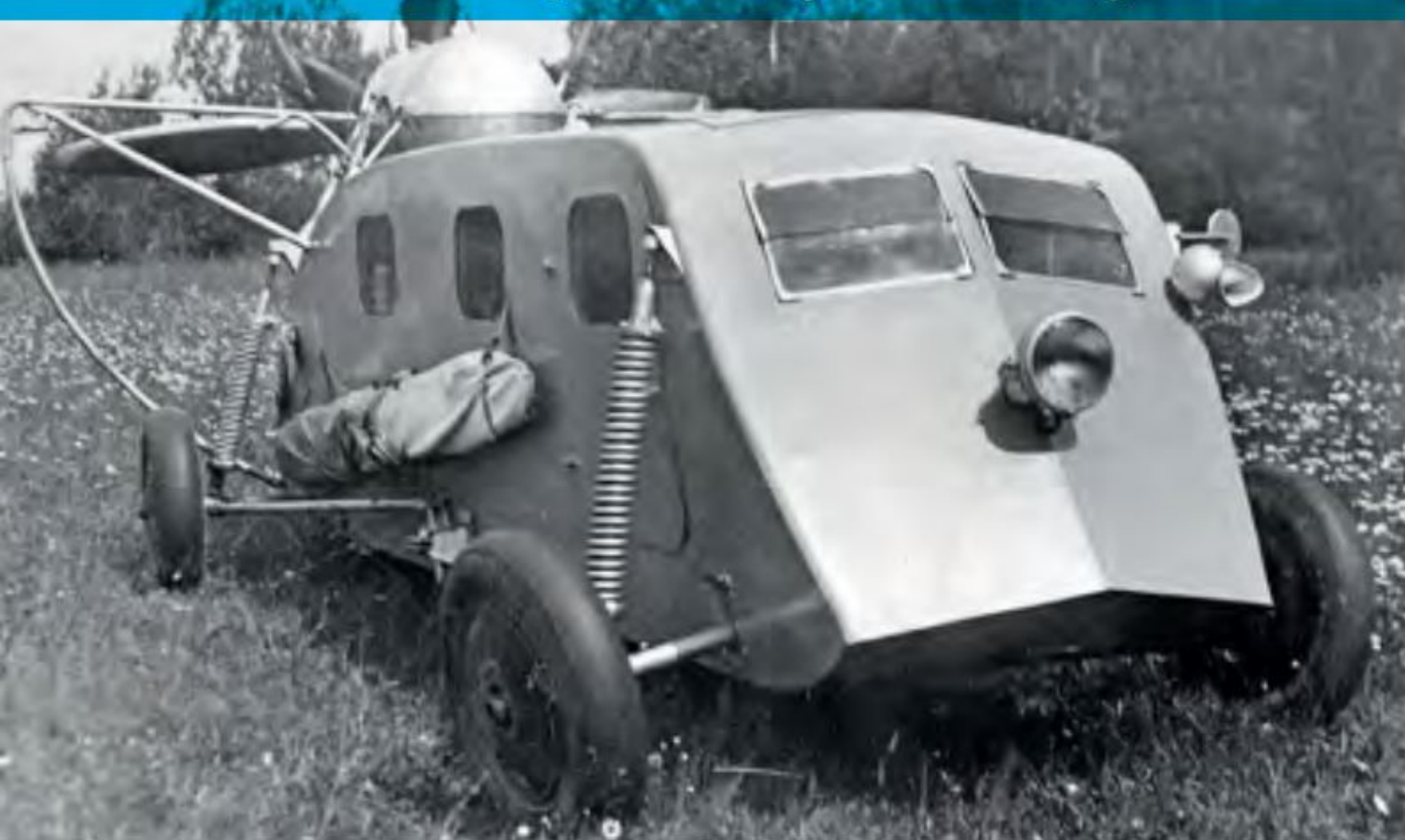
The original NKL-16 M-1942 transport aerosan undergoing acceptance trials at Kubinka in July-August 1942. As the tests were conducted in the summer the vehicle was for obvious reasons mounted on pneumatic tyres for testing. TSAMO
