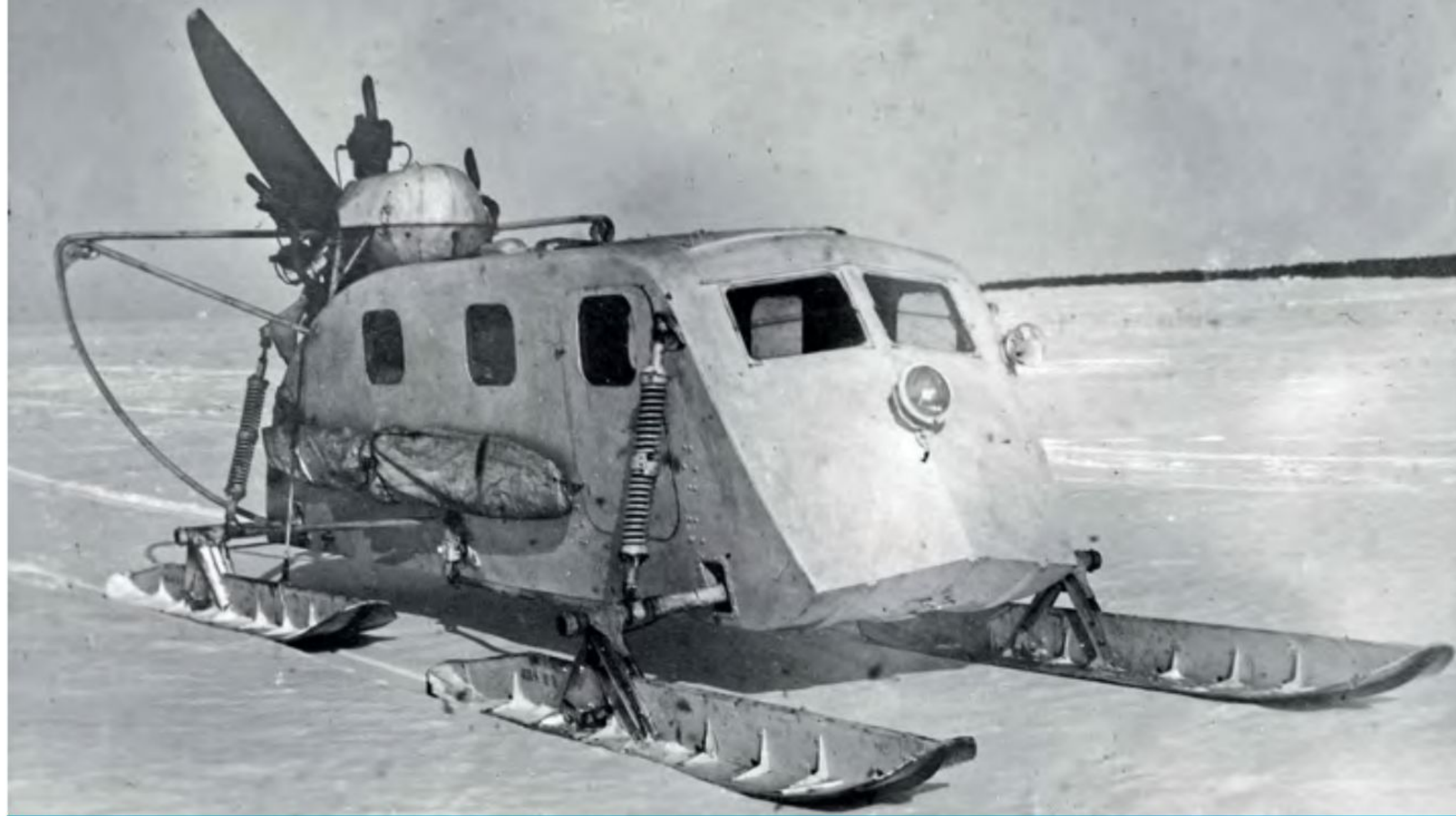
The original NKL-16 M-1942 transport aerosan undergoing trials. Again, note the spare propeller strapped to the side of the vehicle. Aerosans were adept at circumnavigating roads held by enemy forces.
