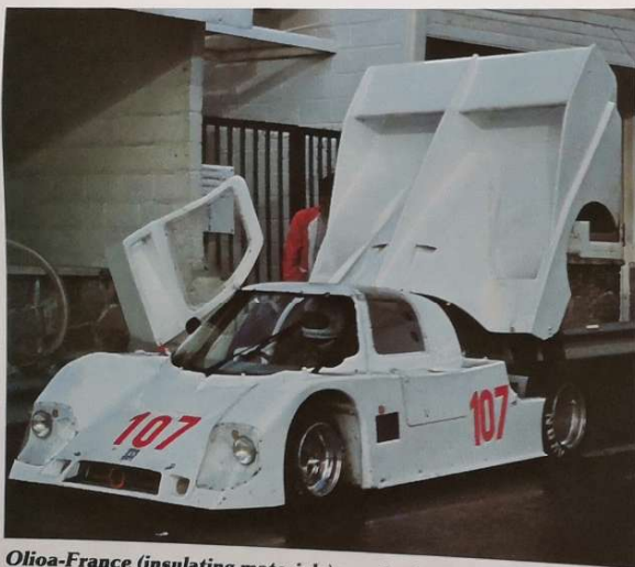
Oliva-France (insulating materials) are the backers of this new C2, the Isolia, powered by a Mader 2-litre BMW, developing 300 bhp for 685 kilos. Perhaps with a fresh coat of paint (not white, please) it will be able to rival with the Spice, Ecosse or Albas.
