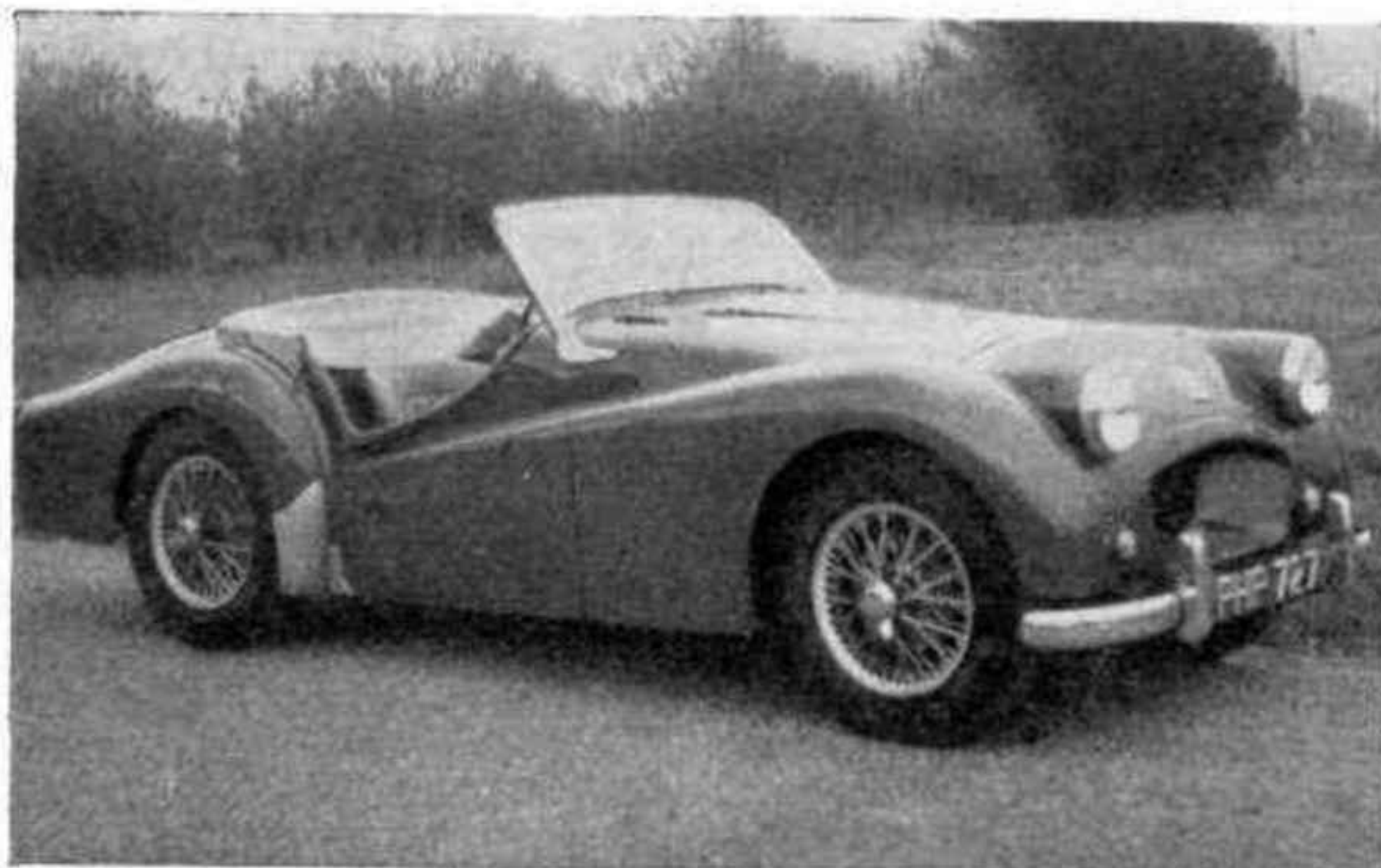
FOR REVIEW. — The Triumph TR2 driven for a four-figure mileage by MOTOR SPORT. It possessed wire wheels, heater and overdrive, and the old-style doors.
