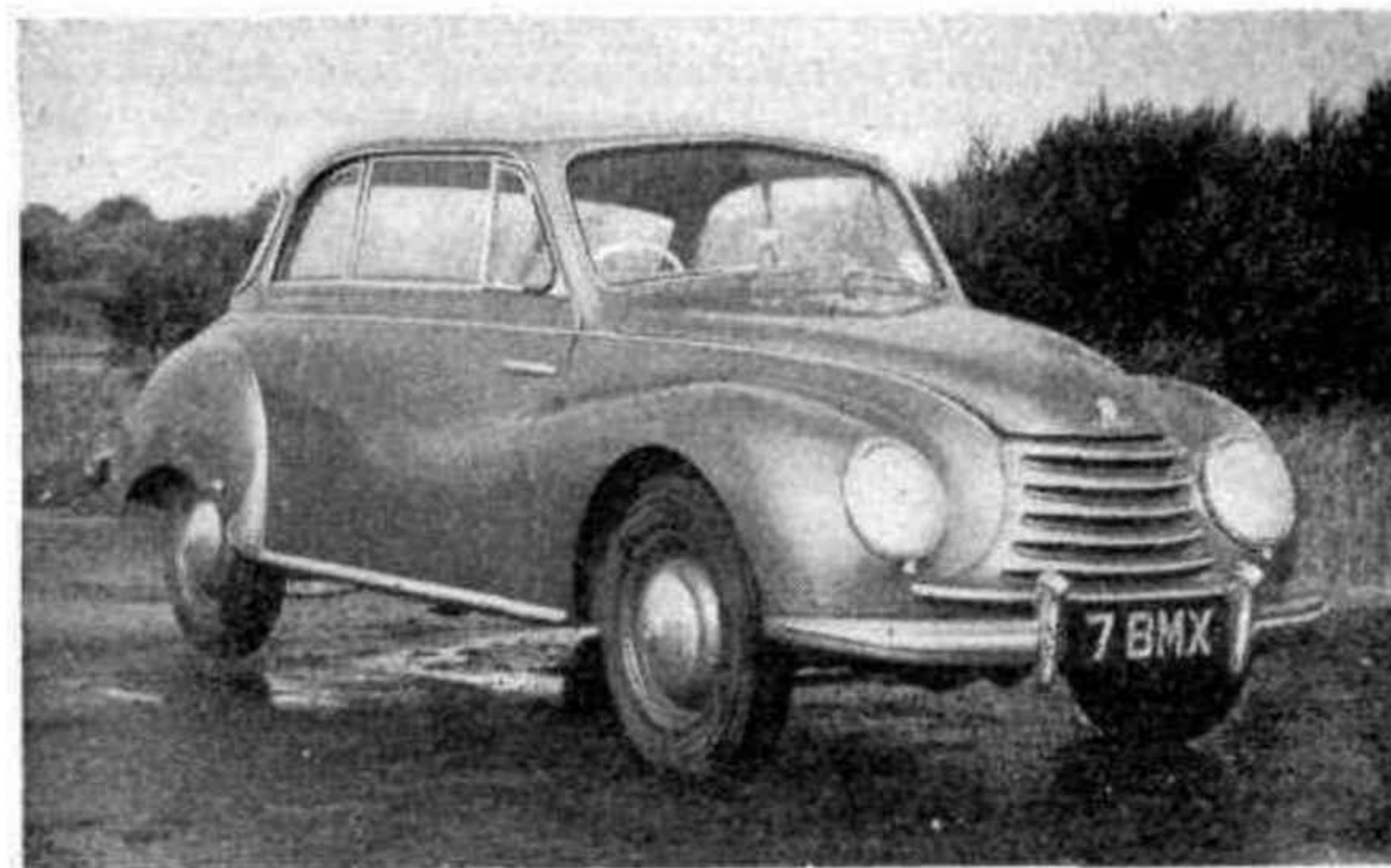
THREE-CYLINDER, F.W.D., TWO-STROKE. —The German D.K.W. Sonderklasse, a small saloon offering exceptional visibility and a surprising performance from its unorthodox 900-c.c. engine.
