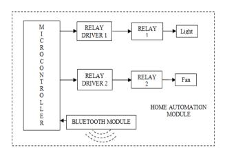
Fig. 2.Block Diagram of Home Automation system
