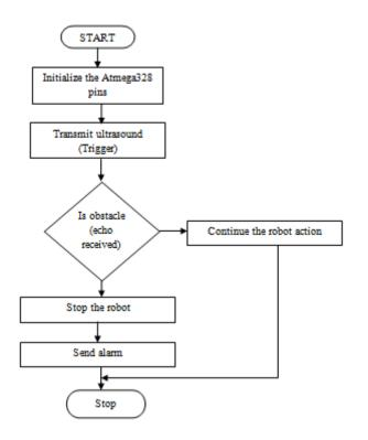
Fig. 8. Flowchart of obstacle detection
