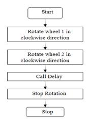
Fig. 4. Flowchart for forward movement
