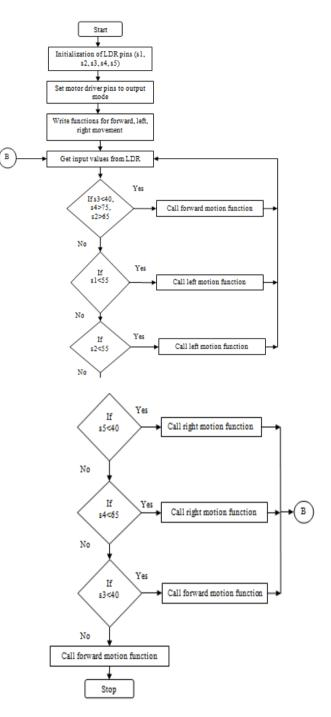
Fig. 7. Flowchart of Line controlled movement
