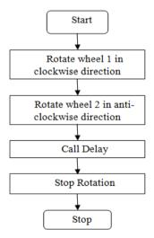
Fig. 5. Flowchart for Left direction
