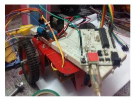
Fig. 10.LED- LDRand wheel Arrangement for line detection
