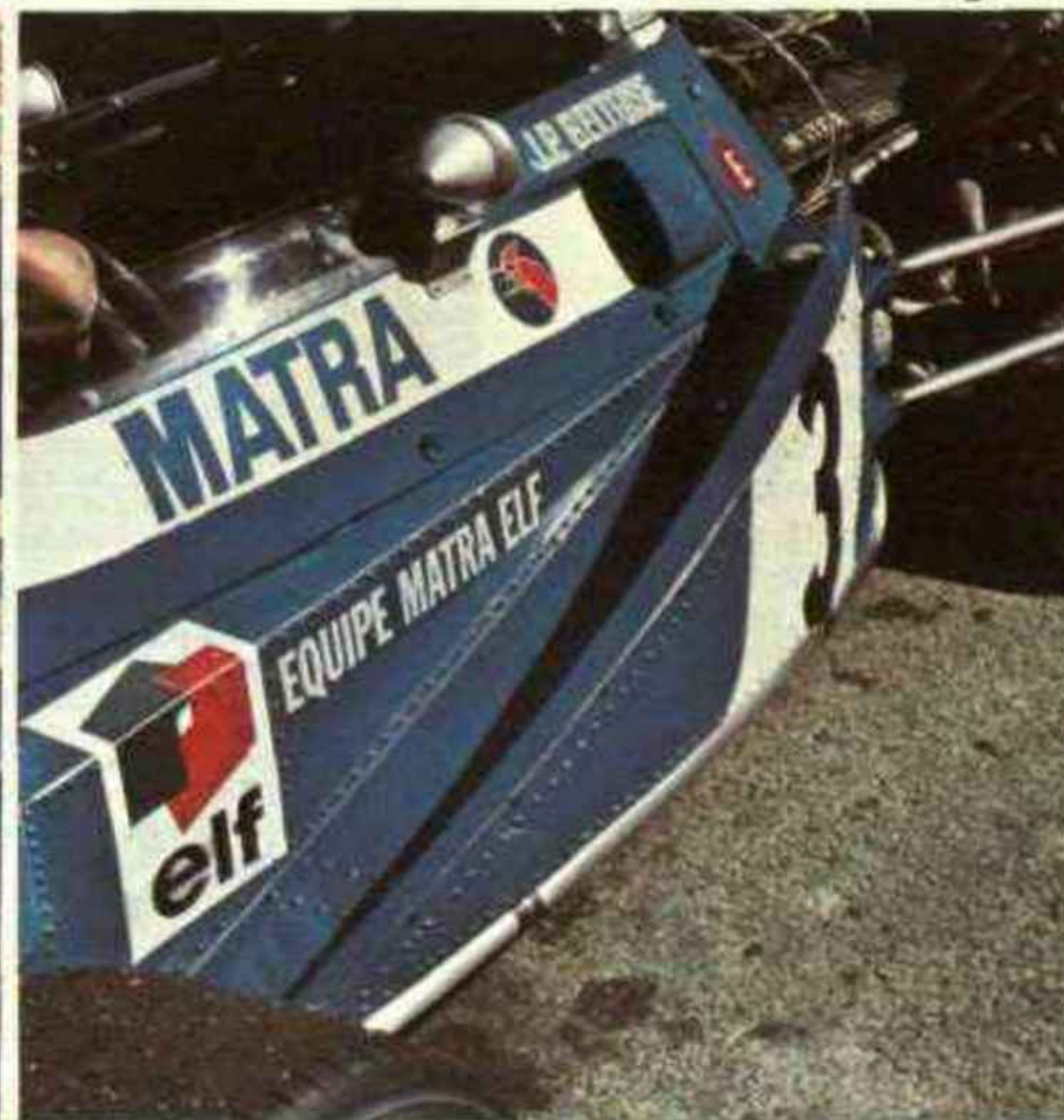
ANGULAR. —The riveted aluminium monocoque of the Matra MS120 presents a strange appearance. The cockpit sides are supposed to present a down-thrust surface and had deflectors attached to direct air onto the engine.
