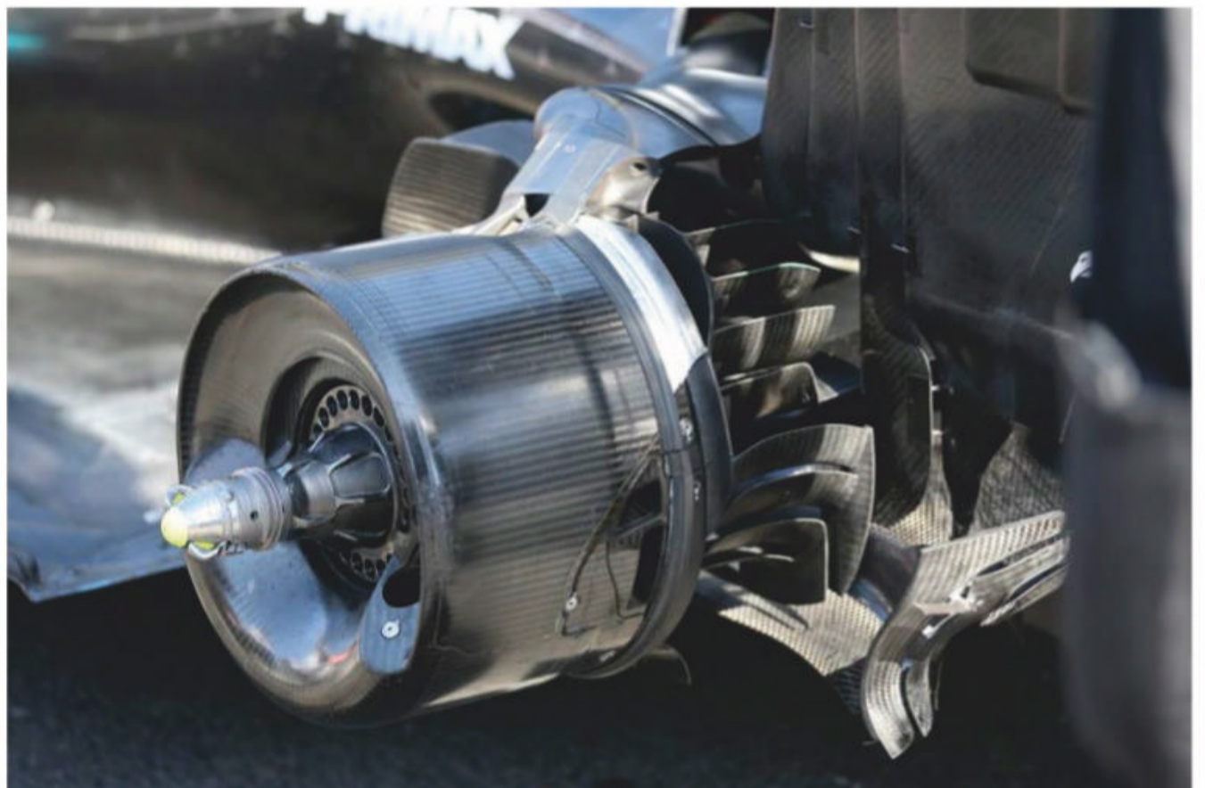
The rear tyres don’t usually require warming up and so teams direct the hot air from the brakes out of the rear brake ducts that are located inboard of the wheel. There are also various outlets within the carbon shroud to allow the hot air to escape
