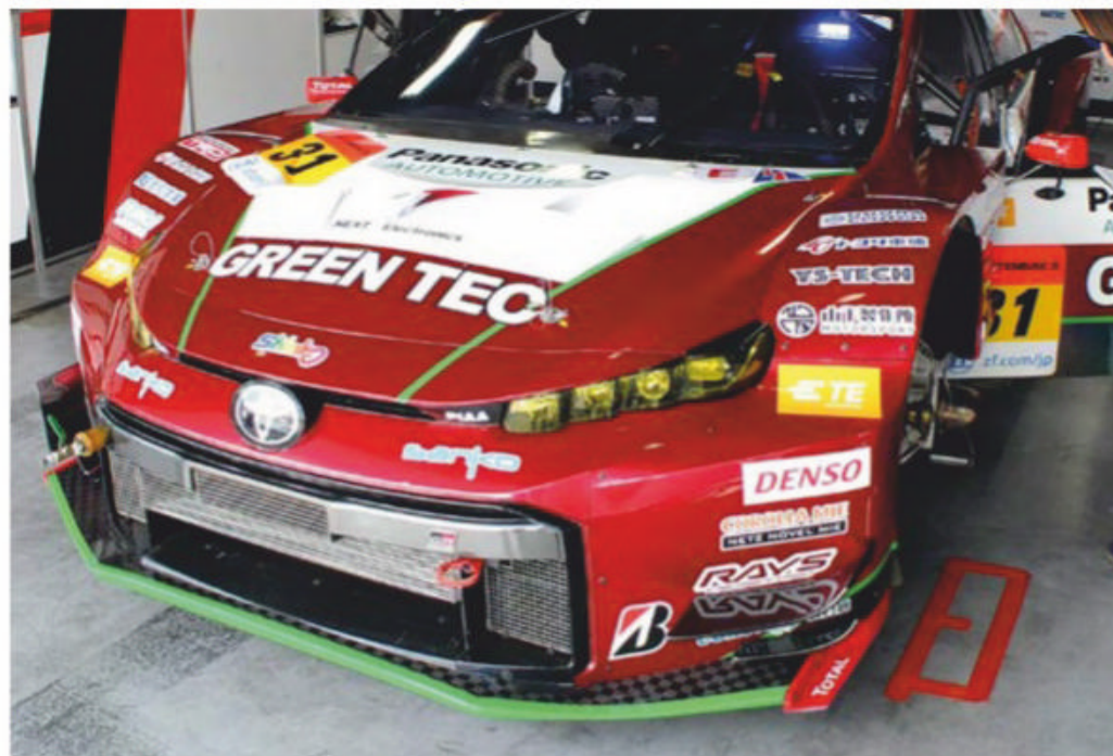
Cooling layout sees hybrid and combustion engines cooled from nose-mounted radiators, while the transmission and A/C system are fed from the rear bodywork
