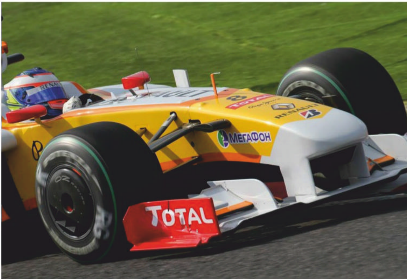
Wheel covers such as those used in 2009 are likely to re-appear in 2021, making arguments about car identity from the wheel design perhaps a little less valid. Note the OZ Racing branding on the wheel cover and holes for heat management
