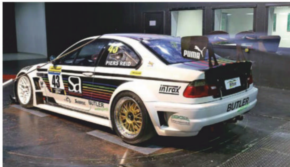
Despite lacking a flat floor and rear diffuser, aero performance was very respectable
