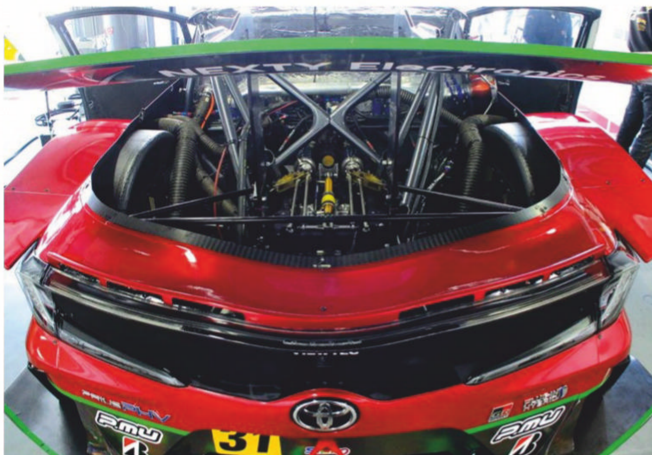
Rear-end layout uses triple dampers with pushrod actuation mounted on top of the Hewland transmission
