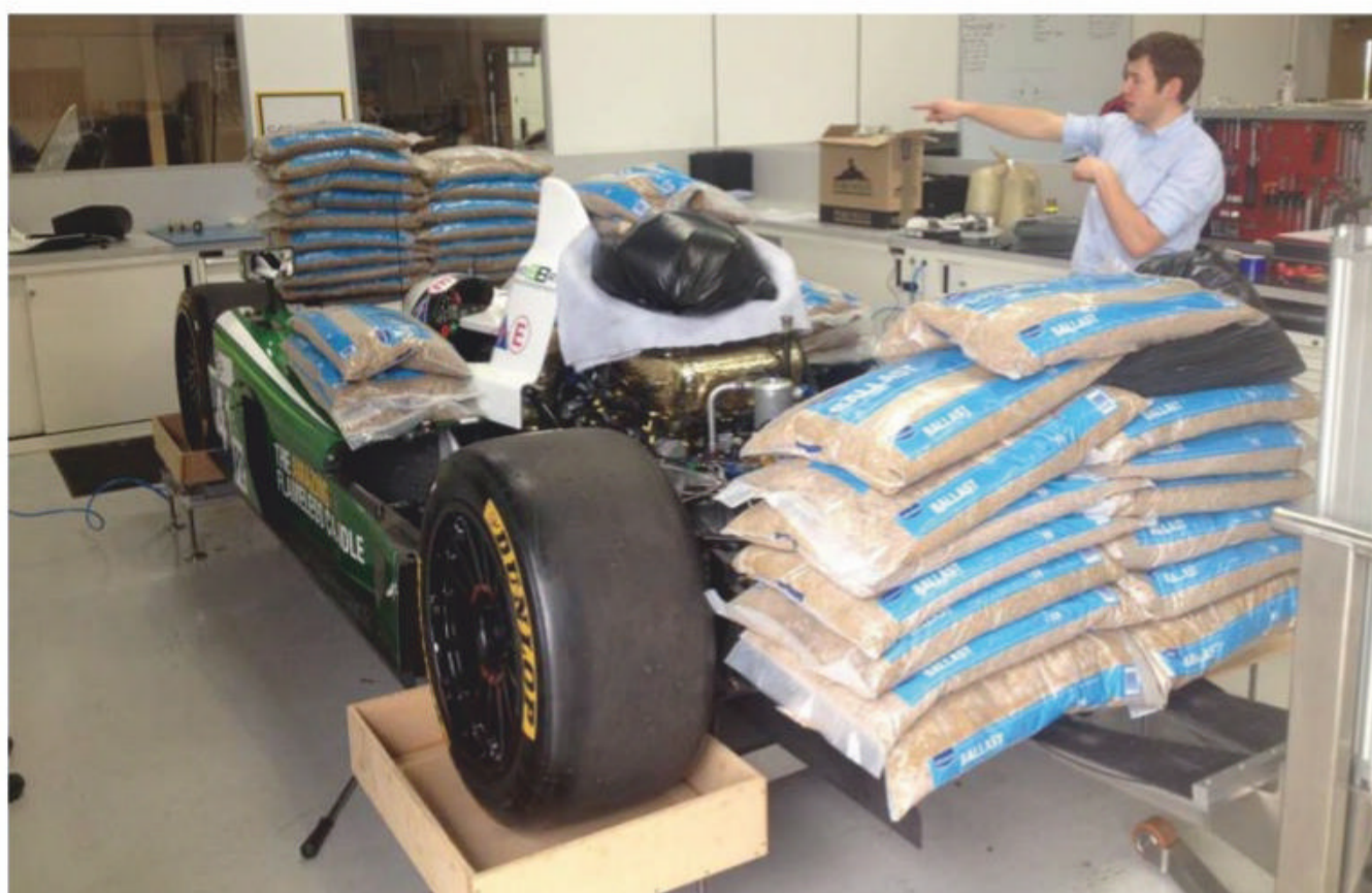
LMP2 pushrod calibration, with a 2,500kg load on the platform. Always best to check the weights before you start
