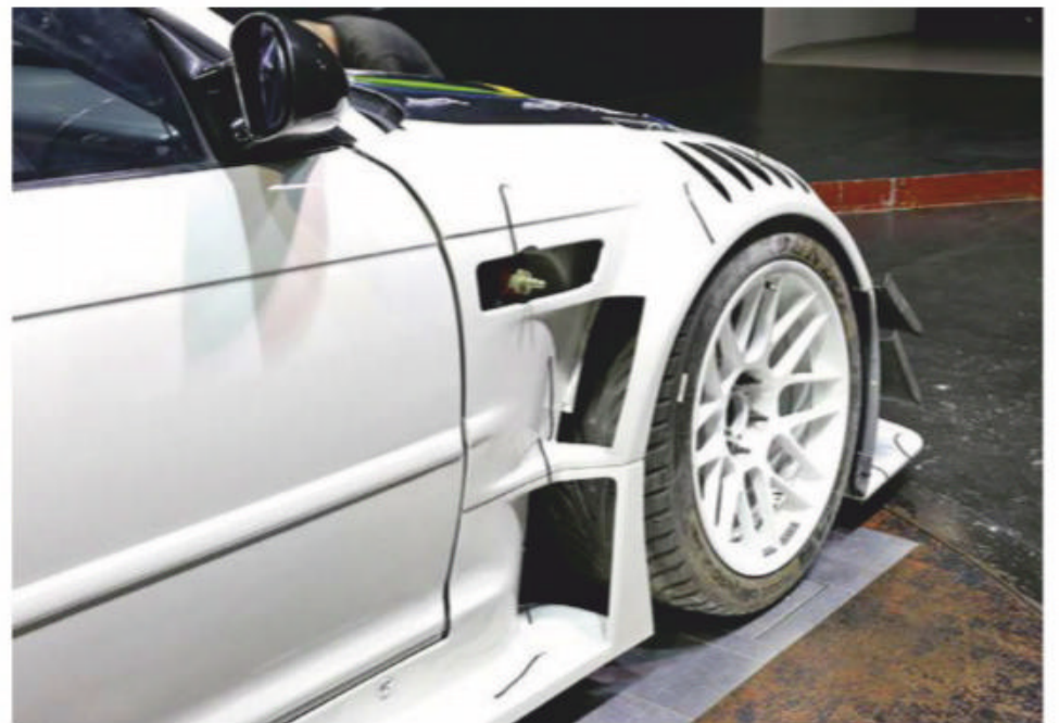
The front wheel arches were vented on top and at the rear in order to help excavate air
