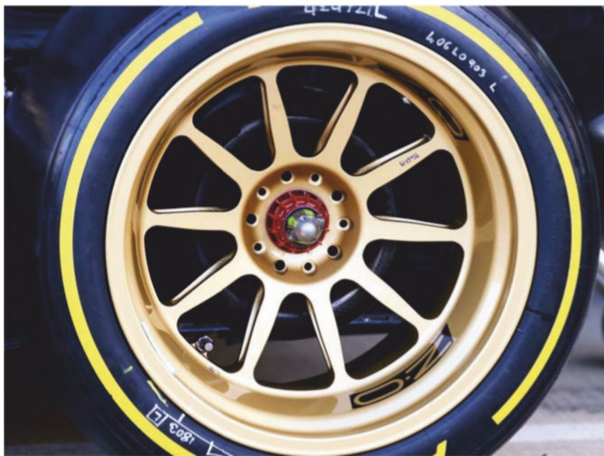
Eighteen inch wheels have been on the cards for a long time, with the first track tests taking place in 2014. As a result, few expect the rims to become a spec part in 2021. It has still to be proven that this will save money
