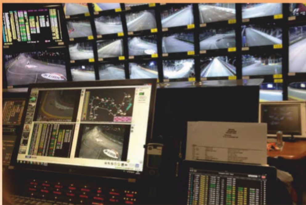
Usually there is a full line of sight around the track due to 30 or so cameras. RaceWatch uses the cars' GPS to switch the cameras to follow each car. This is particularly useful for teams lower down the grid whose cars are often not featured on the main video feed
