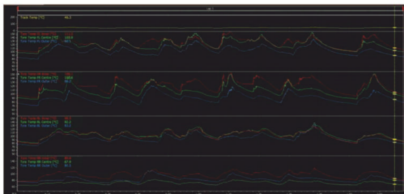
Figure 4: Use gates to bracket displays (here tyre temps) to see if things are working in the correct operating window
