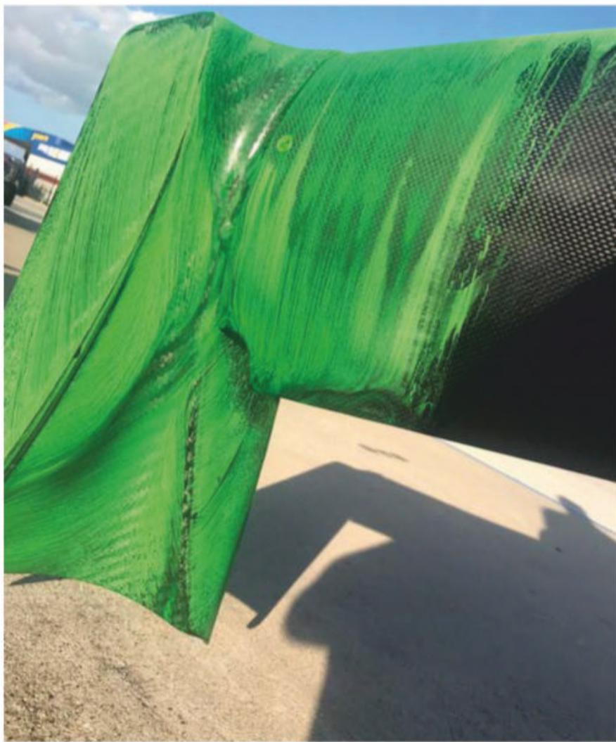
Figure 3a: Surface flow of 2019 notch wing from testing
