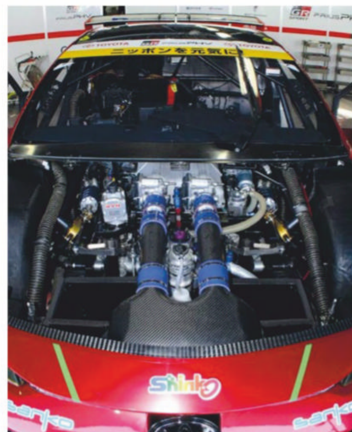
Squeezing the large V8 under the bonnet of the Prius was tough, but apr did it with less than a millimetre to spare
