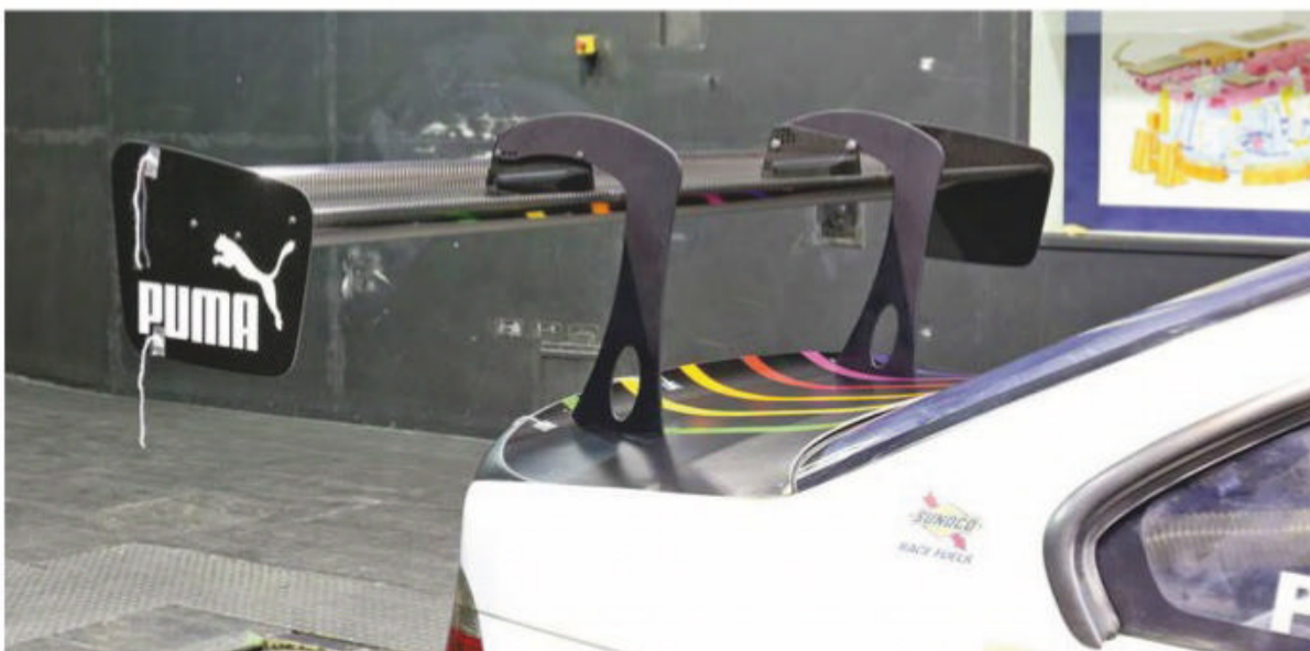
Top-mounted, single-element, well-cambered rear wing with swan neck supports, overlapped the boot spoiler
