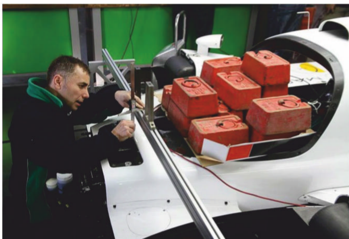
LMP1 with weight load. It is possible to calibrate items out of the car, but best results come from in situ tests
