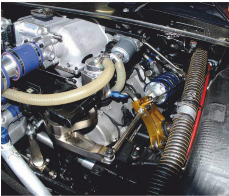
Packaging the front suspension around the engine was a major headache
