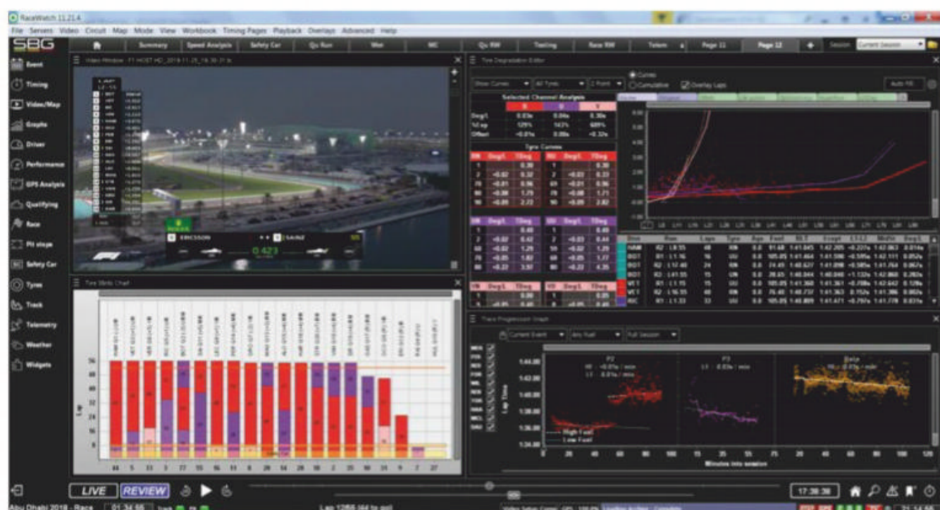
Calculating the degradation of your tyres, as well as those of your competitors, is key to defining the optimum strategy. Tyre degradation is sensitive to changes in car balance and pace, as well as ambient/track temperatures, so requires monitoring
