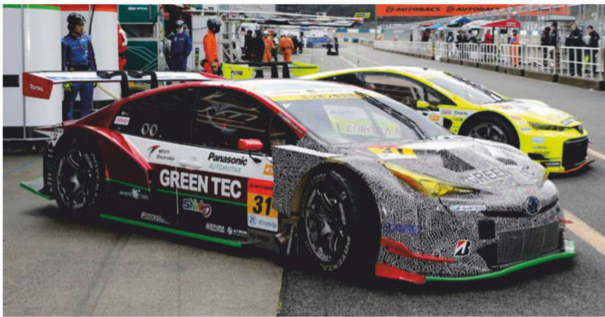
Back-to-back testing was done with the final Prius PHV GT300 (in yellow, behind), and this interim version (front), which used modified 2018 bodywork as well as the 2019 updates shown by the red parts
