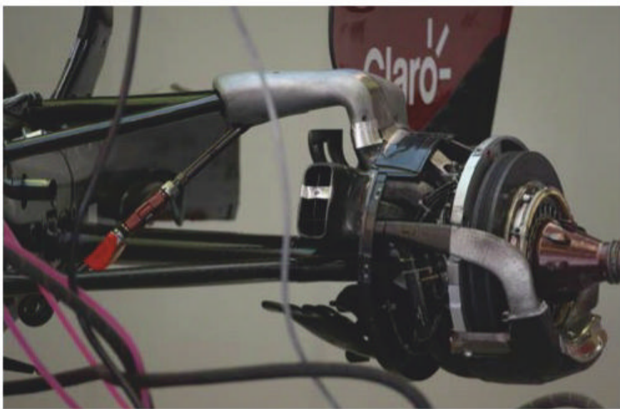
Cool air is channelled from the brake duct inlet down towards the caliper which is clearly shown on the rear of the Alfa Romeo at Barcelona (left) and the Haas at Melbourne (right)
