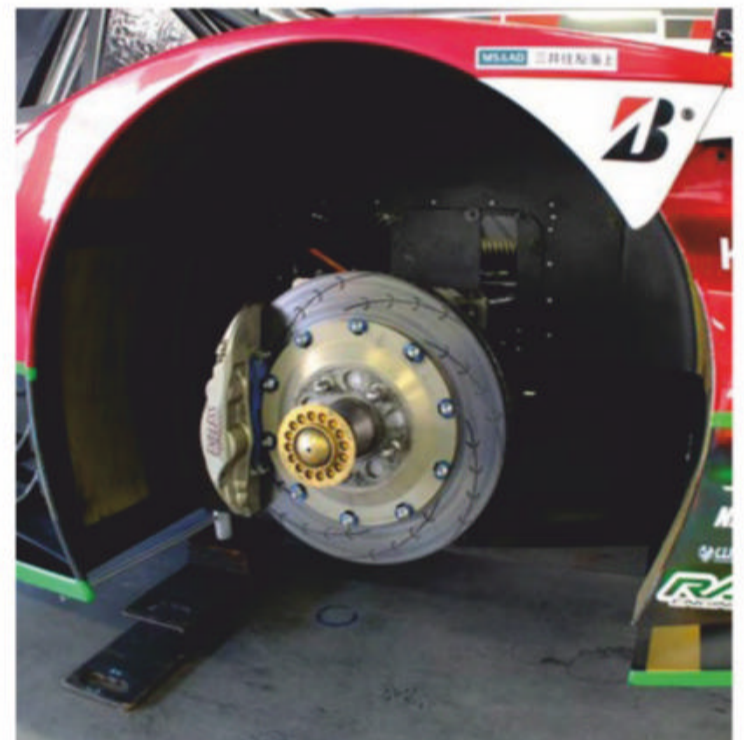
Single-caliper rear brakes are from Japanese company Endless. Twin-caliper set up was abandoned after testing on GT300 Prius
