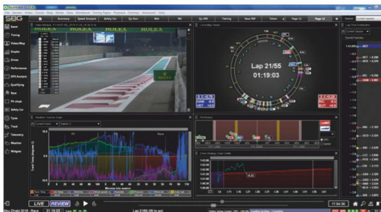
RaceWatch is a software package from SBG that combines all the vital information for a strategist on one screen, together with the live video stream, while also adapting the displays to the context of the race
