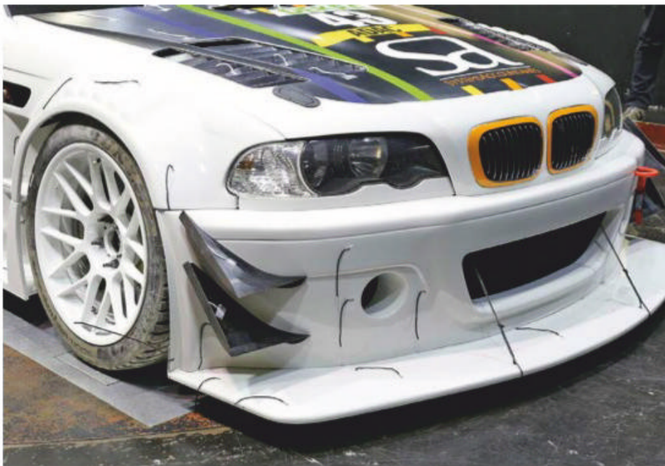
Big splitter with diffusers, dive planes and bonnet louvres all helped front-end aero
