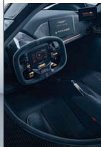
Detachable steering wheel incorporates the Aston Valkyrie's main controls
