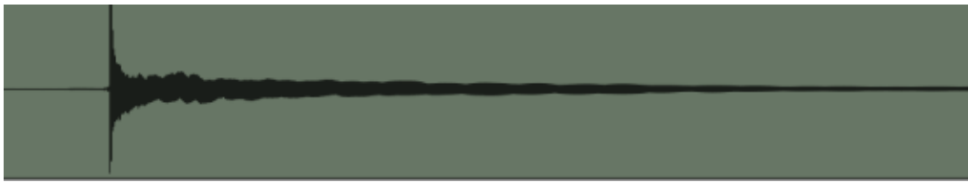
Fig. 8. With a slow attack, the compressor effect doesn't take hold until just after the attack transient. Then the sustained part of the sound is compressed, until it falls below the threshold. At that point, the compressor doesn't just stop working suddenly, it eases off gradually. The result is much smoother, and the attack transient sounds natural.
