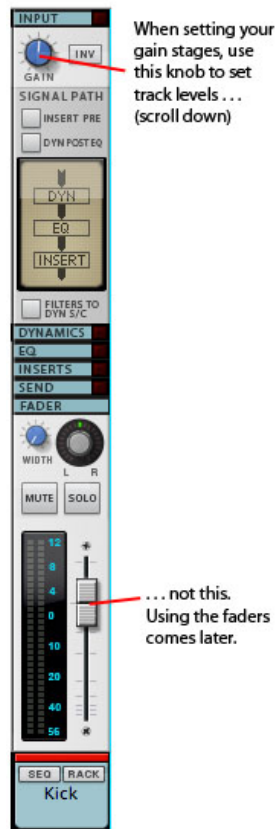
Fig. 6. The gain knob or trim control is often way at the top of each channel on your mixer. In Reason, it's waaaaaaaay up there. Keep scrolling, you'll find it.
