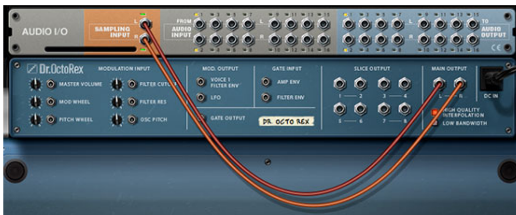
Figure 4: Routing Reason devices to the sampling input is this simple
