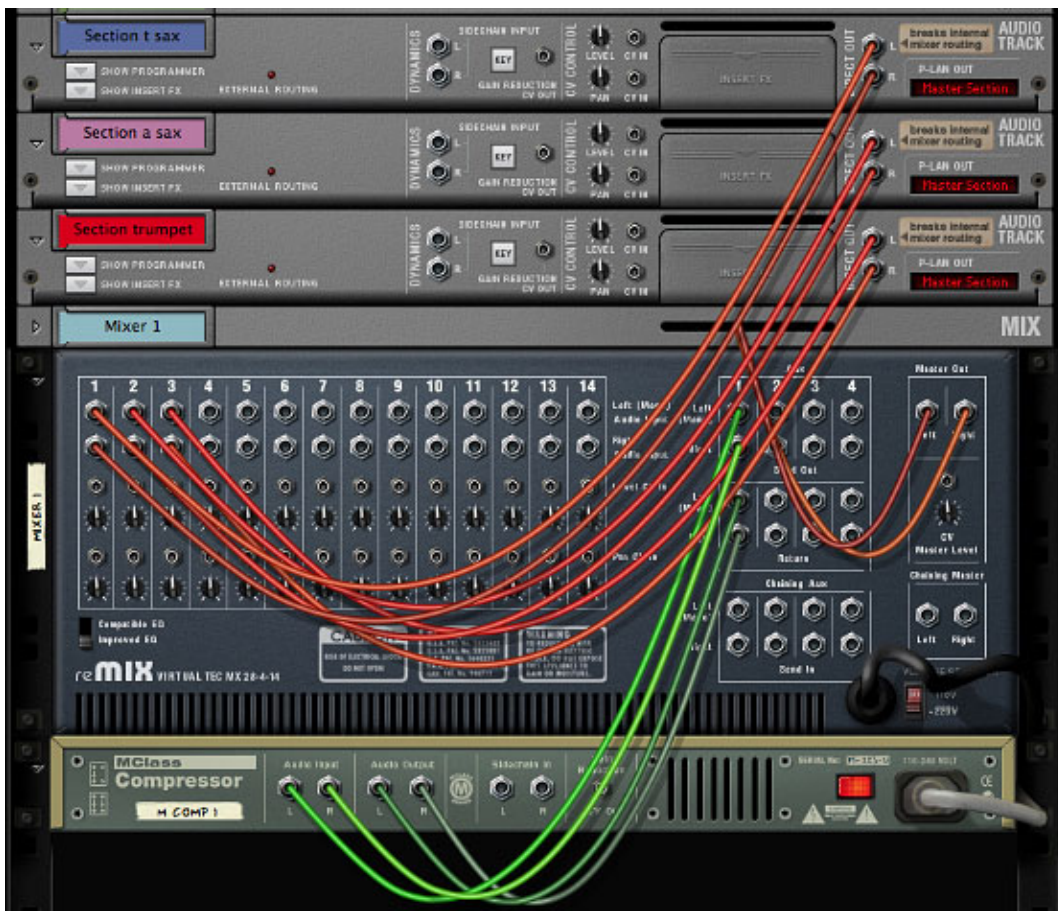
Fig. 12. To set up a background section as a group, add a 12:4 mixer to your rack, then add an MClass Compressor to the rack; the compressor is automatically wired into the aux sends and returns. Then take the direct outs of each instrument or background voice channel, and connect them to their respective channels in the 14:2 mixer. Finally, set all three instrument Aux 1 sends on the 14:2 to maximum, and crank the Aux 1 return above the 14:2's master fader. Now all these tracks can be controlled with one fader, and they all go through the same compressor settings.
