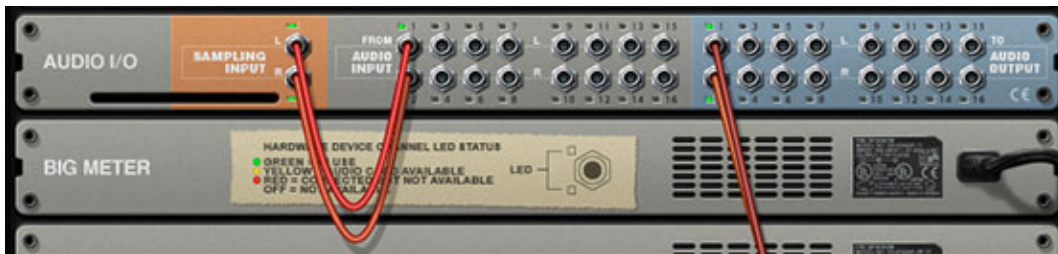
Figure 2: The default routing is Audio Input 1/2 to Sampling Input L/R
