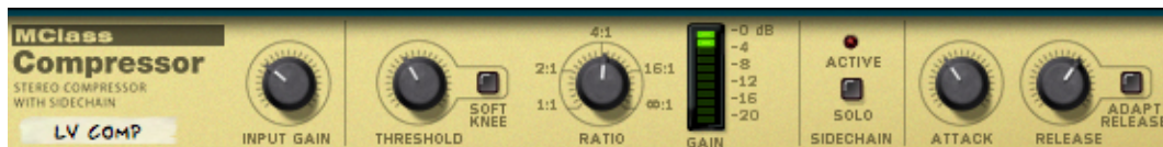
Fig 6. A typical compressor set-up for recording vocals. Moderate attack and release settings ensure a relatively inaudible effect on the input when recording a vocal.
