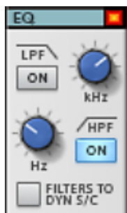
Fig 3. Hi-pass filter in the Reason eq section, set to take out any unwanted noises below 80Hz.
