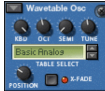
Figure 4: Removing glitches by cross-fading between waves
