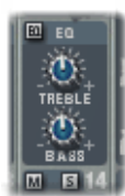
Fig. 13. The two-band EQ on the Reason’s 14:2 Mixer device is a classic example of treble and bass shelving EQ. Turning a knob clockwise boosts the affected frequencies, and turning a knob counterclockwise cuts the affected frequencies.
