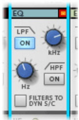
Fig. 21. A low pass filter worked best on these drums; this is the setting.
