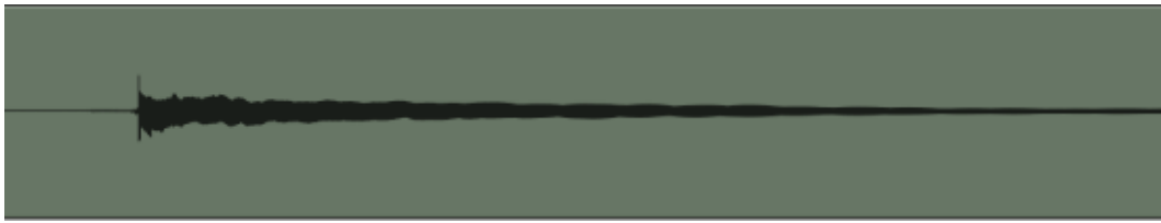
Fig. 7. With the attack and release set for fast response, the attack transient gets compressed right off the bat, as does a portion of the sound that follows the transient. When the signal dips below the threshold, the decay actually seems to jump up slightly in volume.
