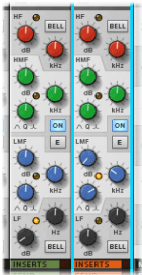
Fig. 20. These are the low mid frequency EQ settings for the organ fills on the right, and the low filter shelving settings for the tenor sax on the left.
