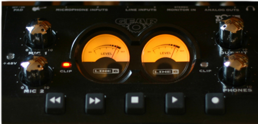
Fig. 2. Many audio interfaces have a simple LED to indicate clipping, as on the Line 6 Toneport KB37; here the left channel clip indicator is lit, indicating clipping has occurred. Bummer.
