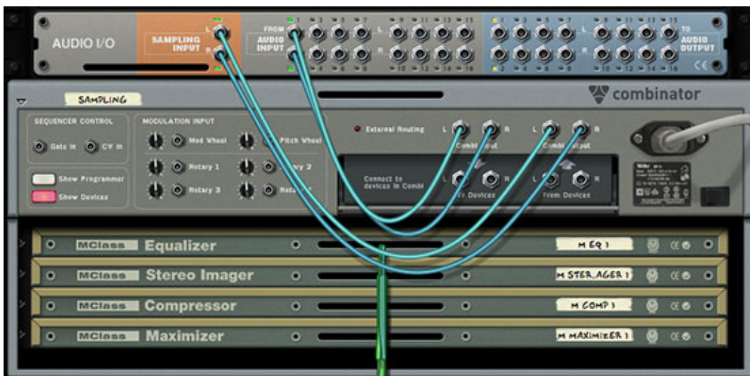
Figure 3: You can process your audio input prior to sampling, for example with EQ
