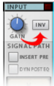
Fig. 7. It's small, but it comes in handy! The invert phase control can solve odd track volume problems caused by out-of-phase recording.
