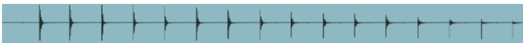
Fig. 10. The only thing that changed for this waveform was that we gradually increased the compression ratio from 1:1 to infinite. As you can see, higher ratio settings can have a dramatic ef-
