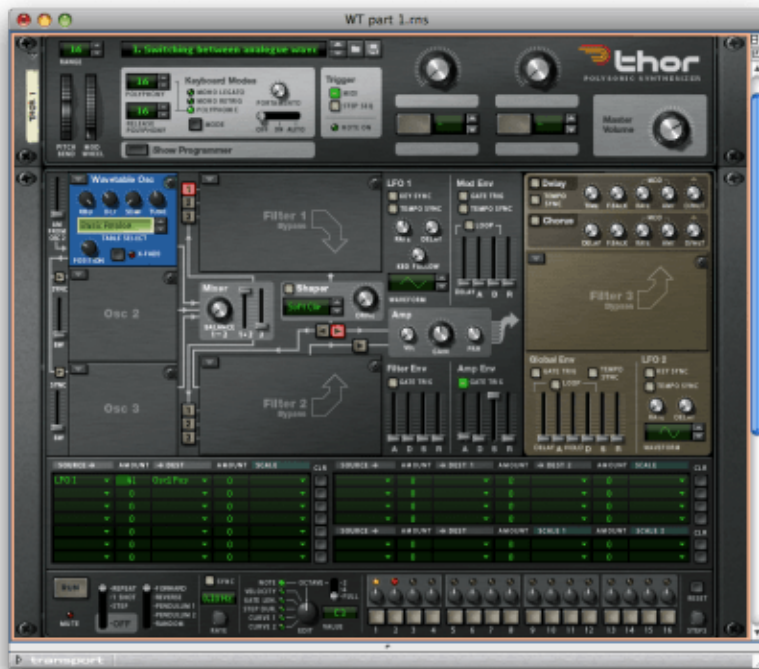
Figure 2: Using an LFO to switch between simple waveforms (Click to enlarge)
