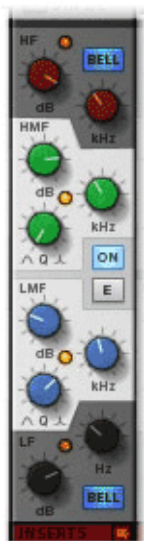
Fig. 16. This is Reason's channel strip EQ, highlighting the parametric EQ.
