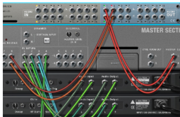
Fig 5. Here we see the back of the Master section where send 8 is routed out of Outputs 3-4 of our soundcard via Reasons hardware interface.
