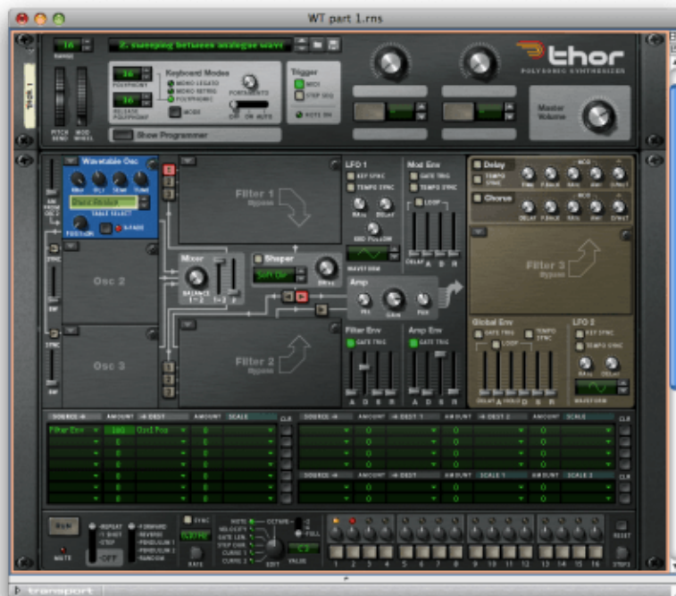
Figure 5: Using the Filter Env to sweep through the wavetable (Click to enlarge)
