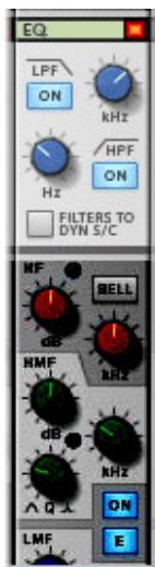
Fig. 11. Reason’s low pass filter lets you set the rolloff point from 100 Hz up to 20 kHz. The angle of the roll-off has particular terminology and characteristics: The angle itself is called the “cutoff” or “knee,” and the “slope” or “curve” reduces the signal by 12 dB per octave. Here you can see how much is allowed to pass at the lowest setting (yellow area only) and how much passes at the highest setting (orange and yellow).
