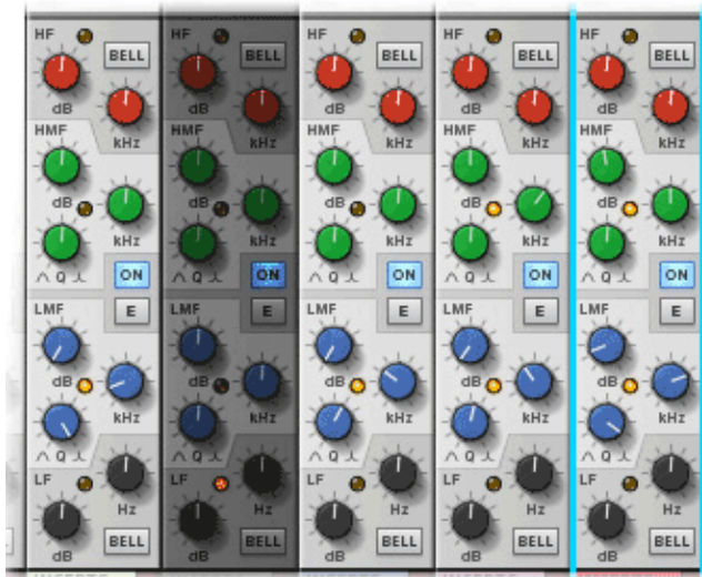
Fig. 19. These are the low mid frequency EQ settings for the guitar, tenor sax, alto sax, and trumpet, from left to right, skipping over the darker channel. The amount of cut is radical, but it's for educational purposes. Plus, it sounds pretty good in the mix, as you'll hear.
