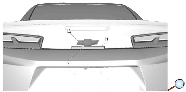
3. Apply masking tape (1), (2) along left side and bottom edge of existing rear bowite (3). This marks where the replacement bowtie will be located.
