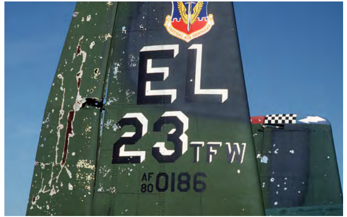
Above left: A-10 80-0186 from the 23rd TFW was damaged by a close detonation from an SA-16 missile. USAF/MSgt Kit Thompson
