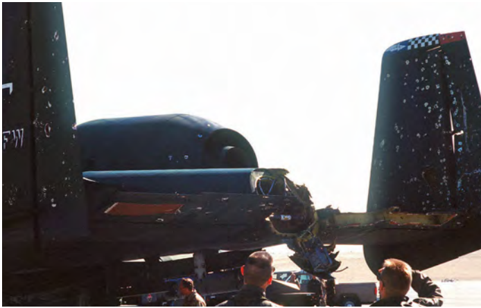
Above left: A-10 80-0186 from the 23rd TFW was damaged by a close detonation from an SA-16 missile. USAF/MSgt Kit Thompson
