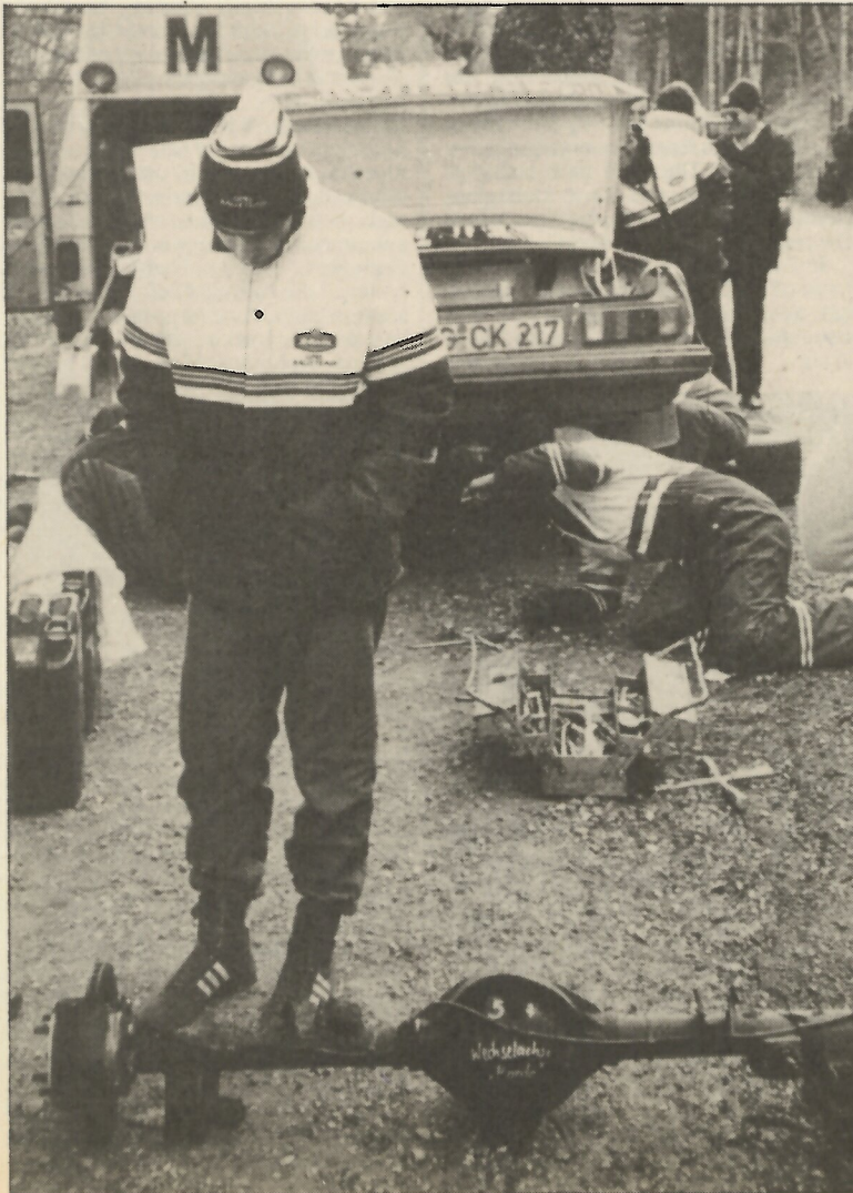
Guy Frequelein reflects on the Opel rear axle which has given so much trouble.
