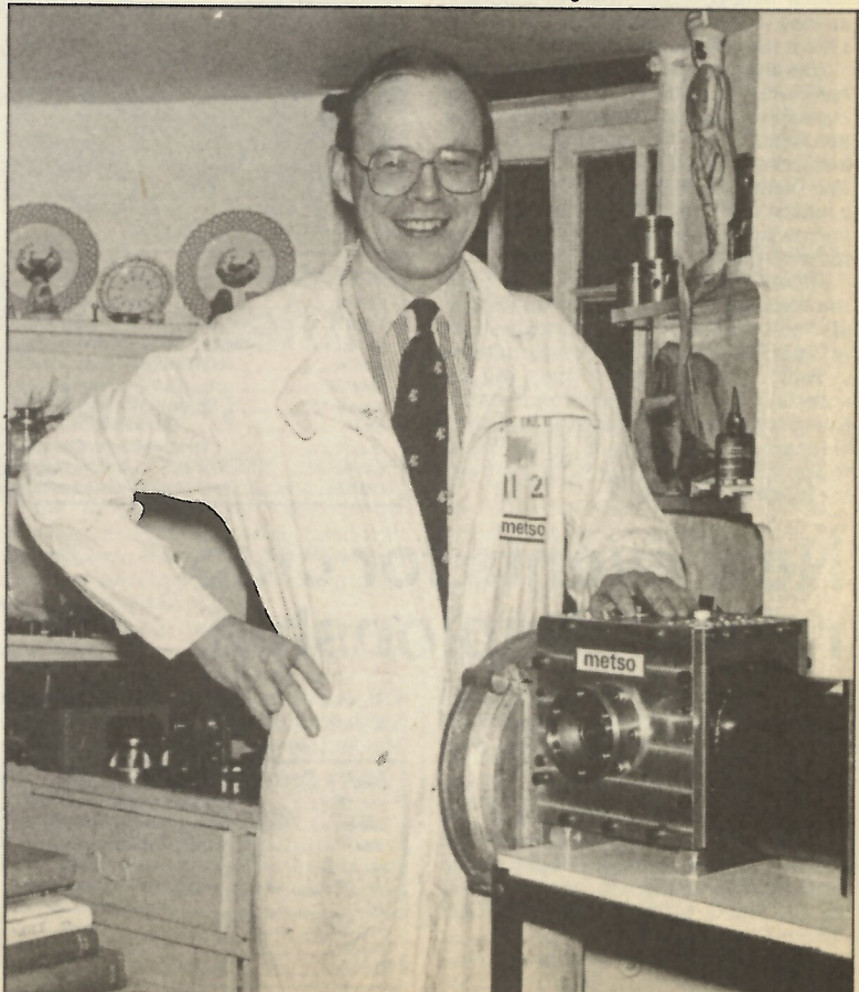
The rectangular differential housing lends the 'box an unusual appearance. Designer Stuart Wallace stands proudly next to his new Metso gearbox.
