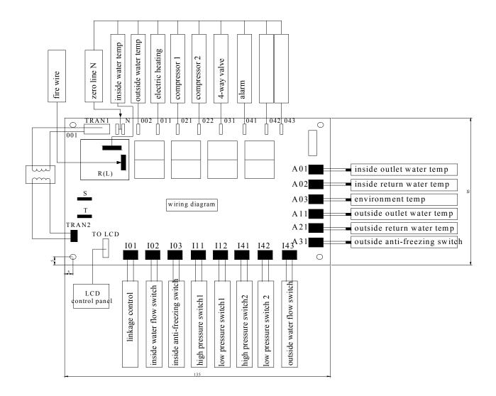
• Don't install the LCD control panels outdoor, please separate the strong electricity and weak electricity when wiring
