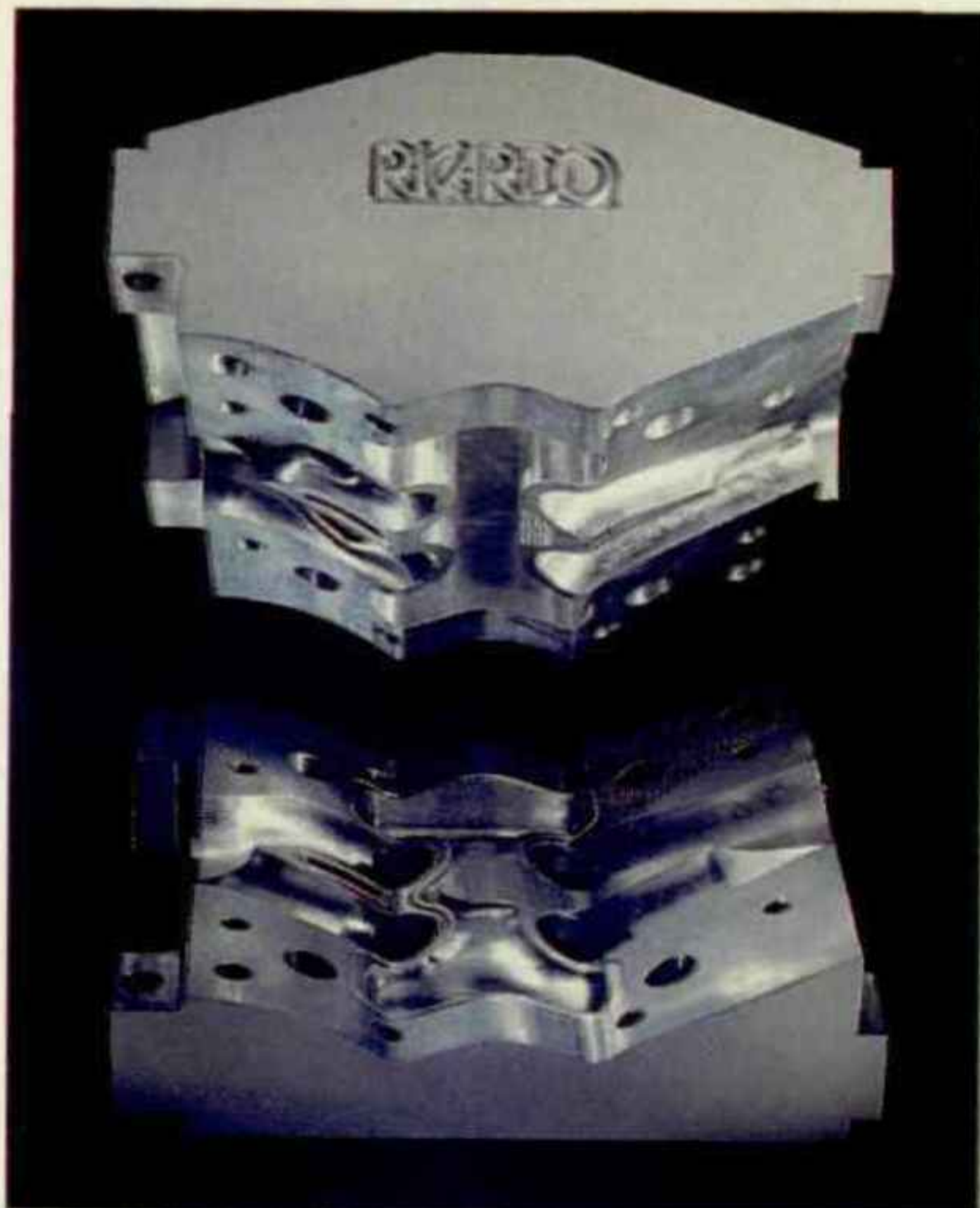
New 3D CAD/CAM development techniques promise a significant reduction in prototype cylinder head procurement lead times, and an improved accuracy of transfer of the developed port shapes to prototype multi-cylinder head castings.
