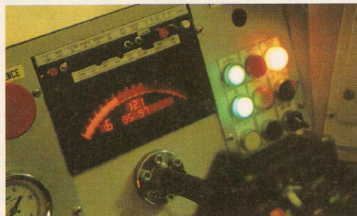
A battery of illuminated panels and different-coloured lights lets the test bed technicians know when to brake and change gear
