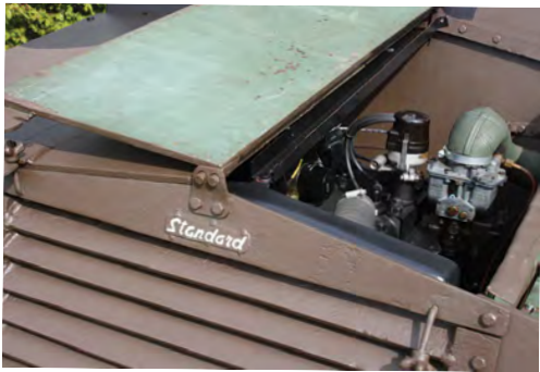
Above: 1776cc four-cylinder side-valve engine is taken from the Standard Flying 14. The Solex carb is specific to the Beaverette.
