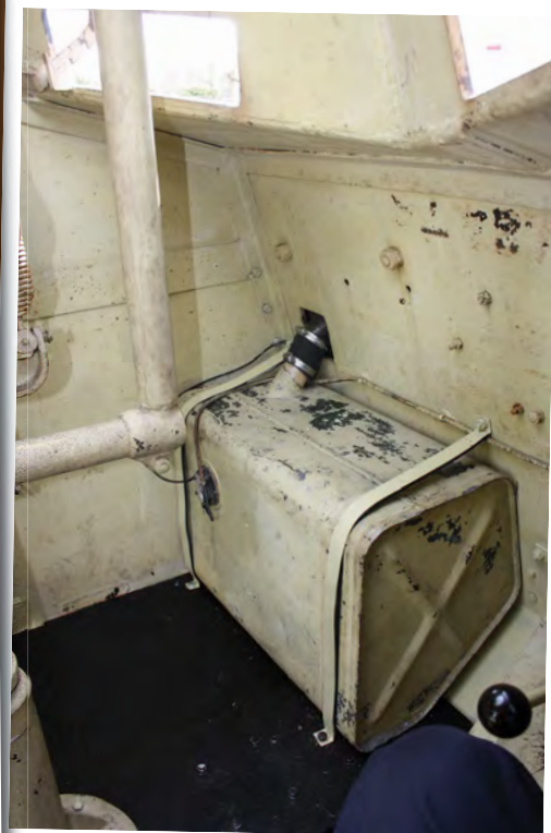
Fuel tank sits conveniently in the front left corner of the cabin.
