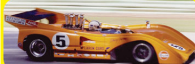
1971 McLaren M8F Can Am car. Ran Kinsler prepared MacKay intake Manifold with Lucas mechanical metering.
