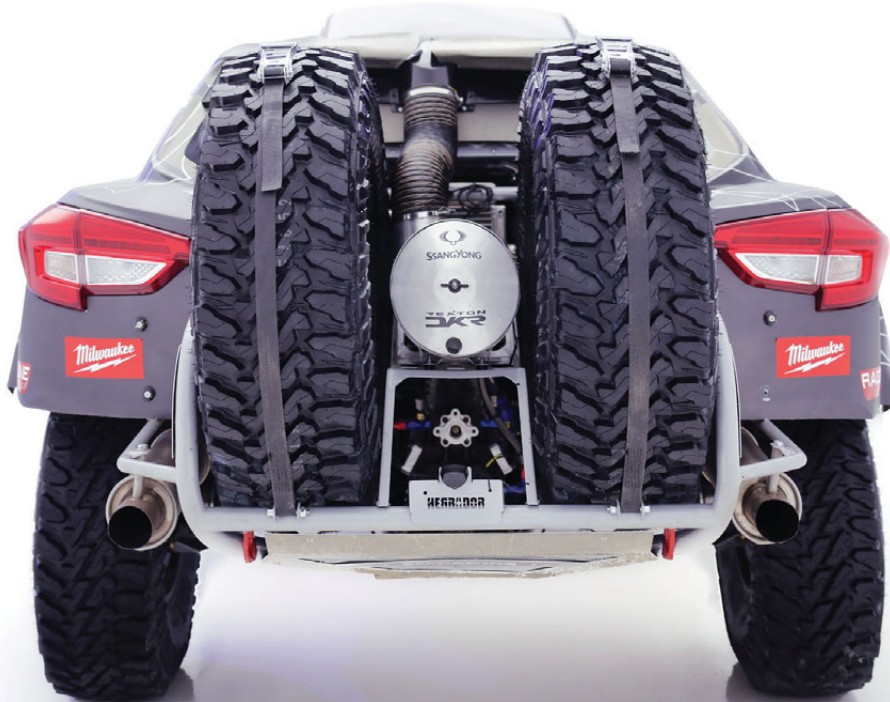
BELOW The spare wheels and 400-litre fuel tank hang out at the rear of the chassis to achieve the preferred weight distribution
