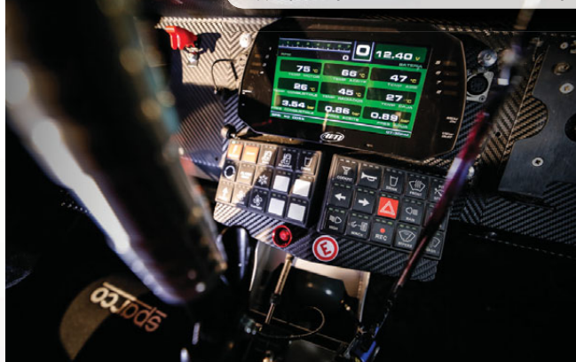
ABOVE & BELOW The Rexton DKR's interior. A new MoTeC programmable switch allows engine mapping changes in real time while eliminating all fuses and relays to enhance electrical reliability
