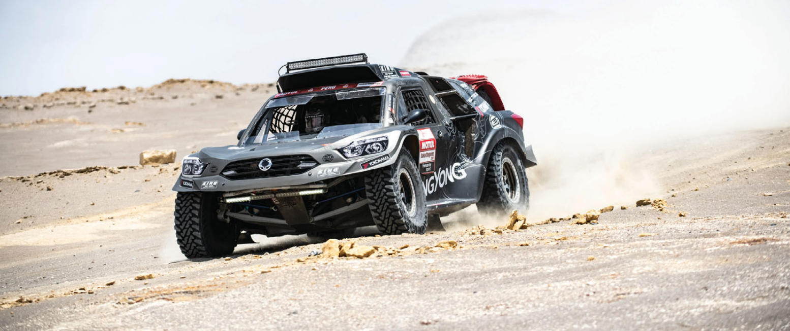
ABOVE & BELOW Greater suspension travel and a weight break are among the compensations for running in two-wheel drive trim
