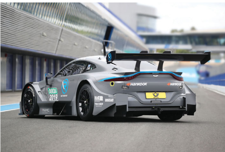
ABOVE & BELOW The first test of the Aston Martin Vantage DTM inevitably threw up teething problems with vibration and temperatures, issues rivals had encountered three months earlier
