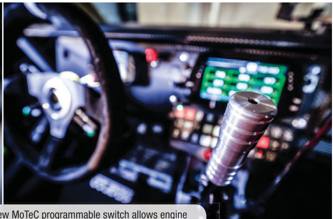
ABOVE & BELOW The Rexton DKR's interior. A new MoTeC programmable switch allows engine mapping changes in real time while eliminating all fuses and relays to enhance electrical reliability
