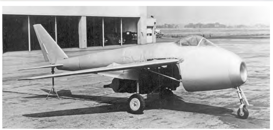
The Messerschmitt P.1101 was designed to have a ground-adjustable swept wing. It would be pivotal in the development of the Bell X-5 – which would be the first aircraft capable of varying its wing geometry while in flight
