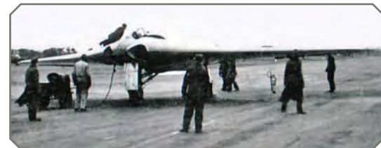
The Horten Ho 229 was designed in response to Hermann Göring's call in 1943 for a bomber capable of meeting the "3x1000" requirement. It was to become the first pure flying wing powered by jet engines
