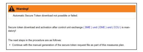
By clicking on the "OK" button, ISTA generates the required TokenRequest\_VIN\_xxx.json file and opens a file dialogue to save it. The file must be sent to technical support later via PuMA or TSARA.
