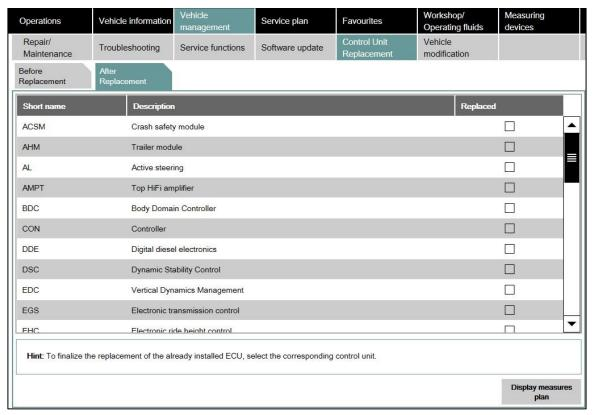
To do so, select the corresponding control unit in the "After Replacement" tab and then execute the measures plan.
