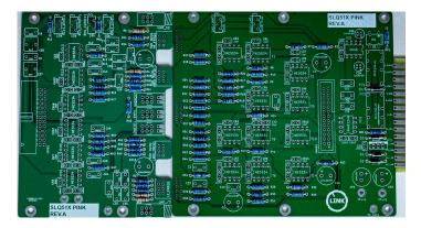
After Placing and Soldering all Resistors, we solder the next bigger parts like IC-Sockets and small Capacitors, like 39x100nF and 18x22pF
