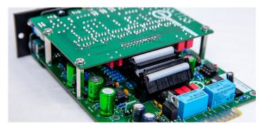
Now we install the upper subboard by holding it angled and connect the ribbon cables at the same time.
