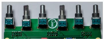
After having one pin of each pot soldered we add the bracket like shown in the picture above. The direction of the bracket is shown in the picture below. After having all pots screwed to the bracket, we can solder all pins, then we need to cut the pins.
