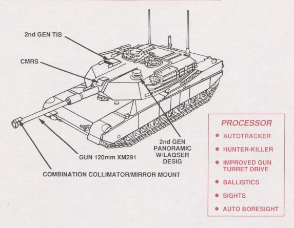
ATAS ATD I: This program initiated in October 1992 will demonstrate the integration of maturing technologies within current Abrams physical constraints and demonstrate increased acquisition, lethality and hit probabilities. Components to be included on an M1A2 Vehicle include the 120mm XM291 Gun, 2nd generation FLIR Technology for both commander's and gunner's sights with an integrated laser designator, autotracking and hunterkiller capability. Demonstration is planned for 4Q FY94.
