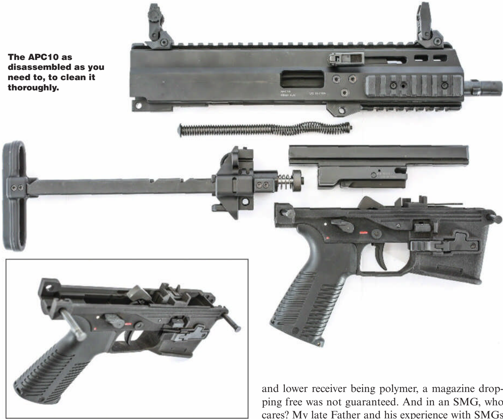
The lower is a polymer housing with the internals held in place by cross pins. Once off, you can dunk it, douse it, scrub it, lube it, and then re-install it.
