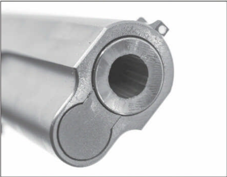
The lack of a bushing means the barrel comes flush to the slide, and this means a deep crown to protect the ends of the rifling. Also, the recoil spring retainer is a reverse plug, installed from the breech end.
