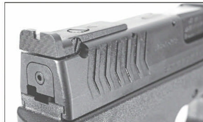
The rear sight is an adjustable one, so you can dial in your 10mm loads.
