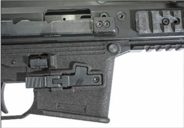
Here you can see the right-side magazine catch, and the lever system to operate it.
