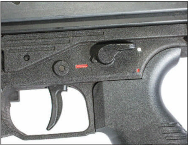
The selector on this one goes from Safe to Semi to Auto, and that means a long list of volunteers for test-firing.
