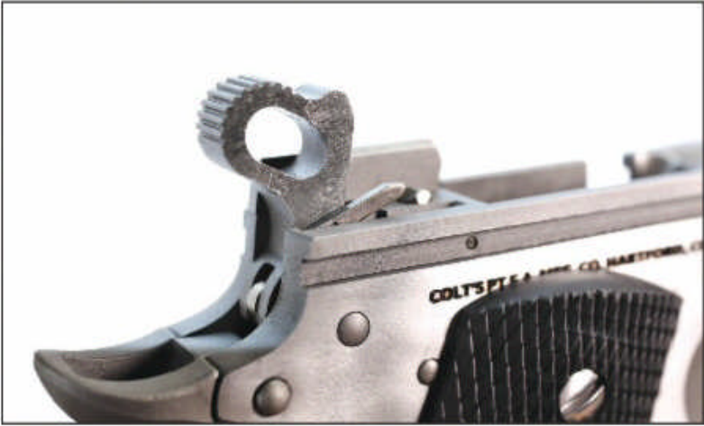
You can see the Series 80 firing pin safety lever here, in its raised position, as it would be when clearing the firing pin for forward movement.
