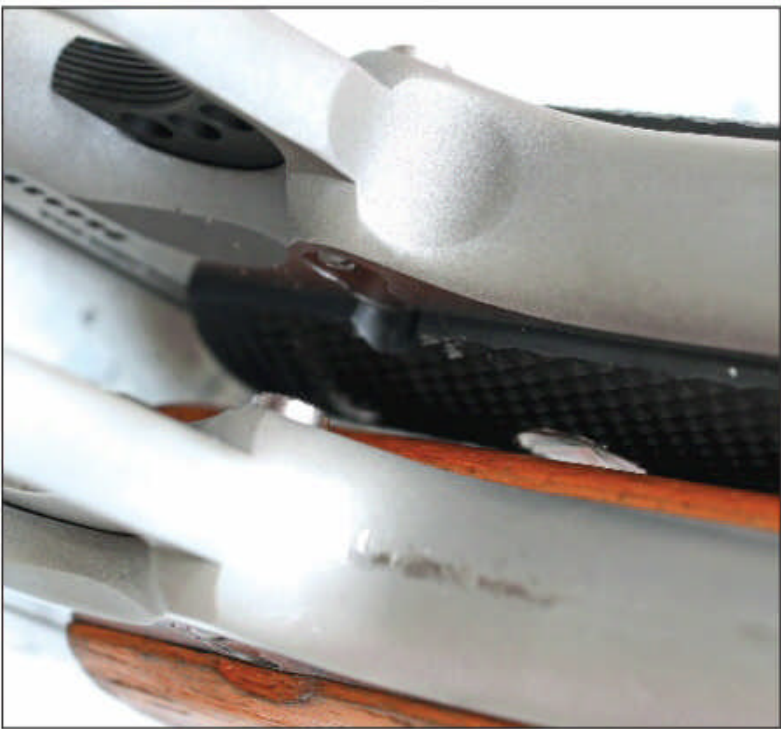
The new Delta, above, has the frontstrap lifted, and the old one is just the way 1911s had been made since 1911.
