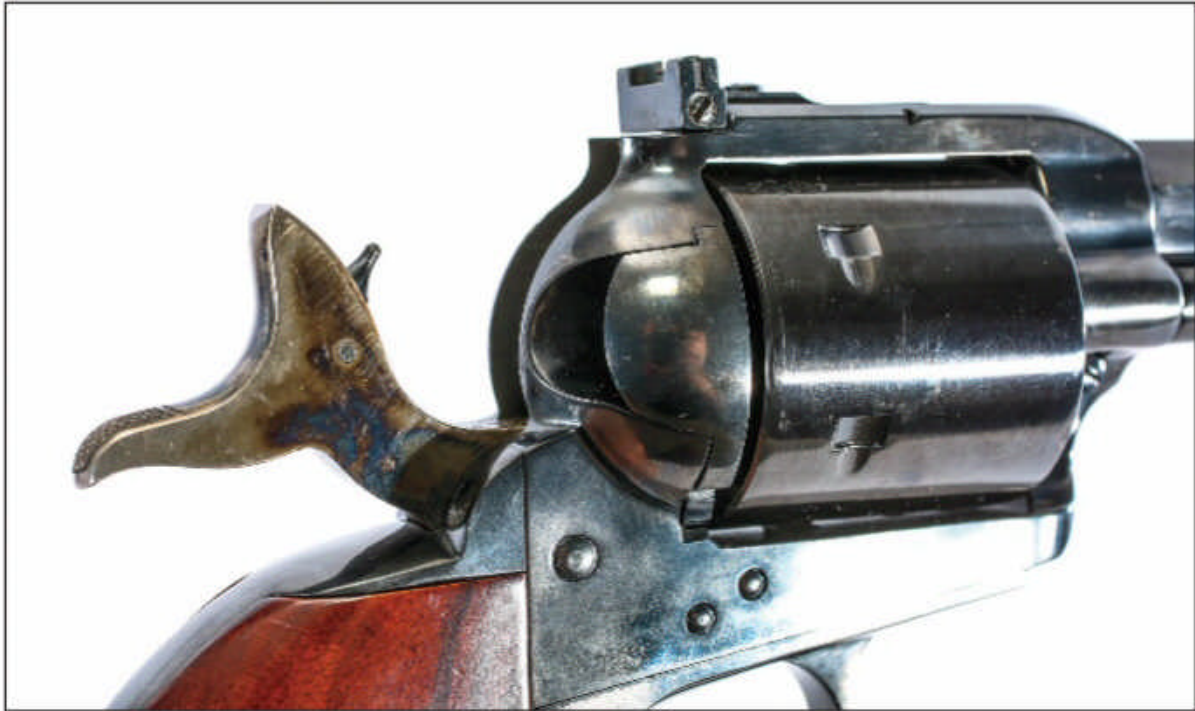
The firing pin is fixed to the hammer and passes through the frame to the primer.
