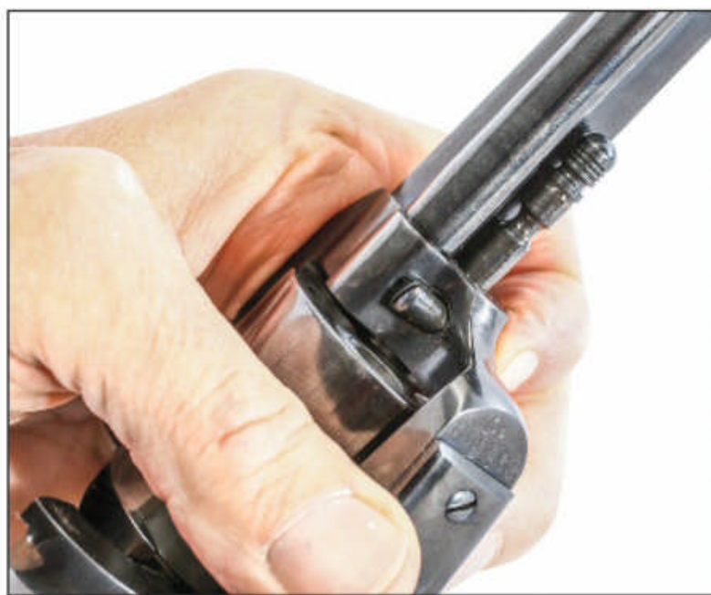
The Cimarron Bad Boy uses the Pre-War cylinder pin latch, a spring-loaded cross pin to hold the base pin in place.
