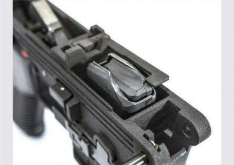
The APC10 locks open when the last shot is fired, by means of the bolt hold-open lever that is actuated by the magazine follower.
