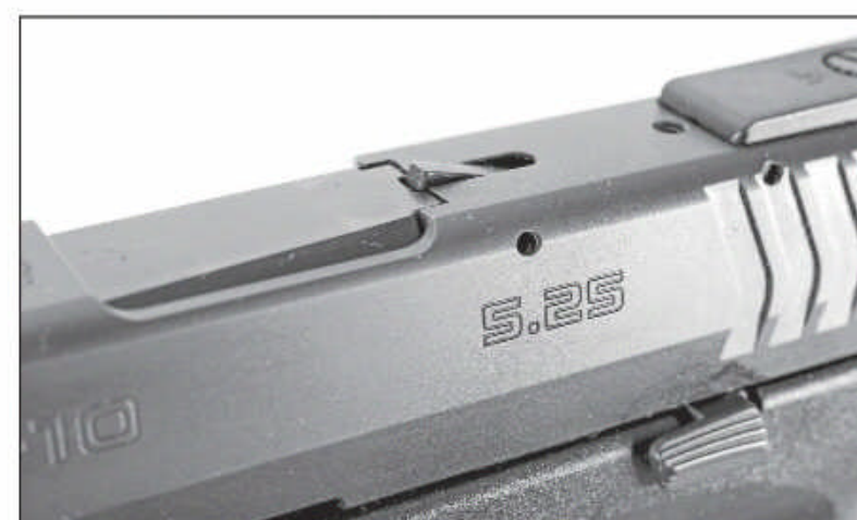
The loaded chamber indicator is easy to feel with a fingertip when there's a round in the chamber.
