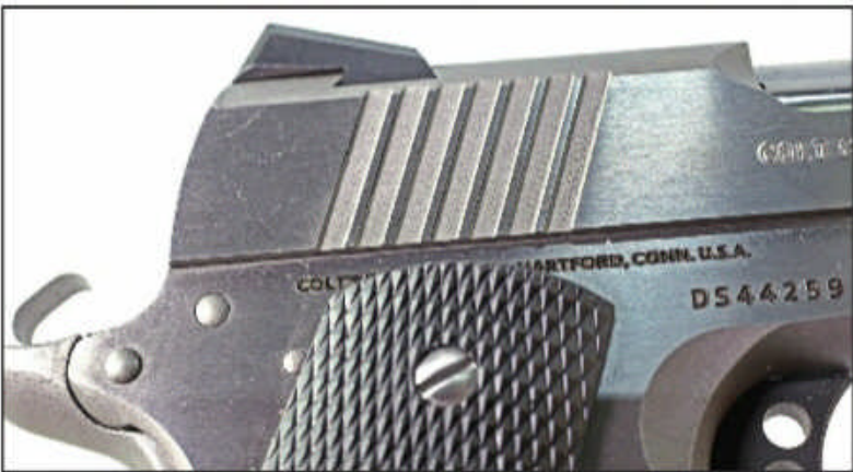
The cocking serrations are seven wide, flat-bottomed grooves angled on the rear of the slide.
