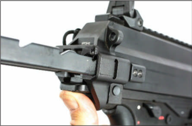
The button underneath is how you extend or retract the stock. Well, you can extend it by just grabbing and yanking, but it won't collapse the same way.
