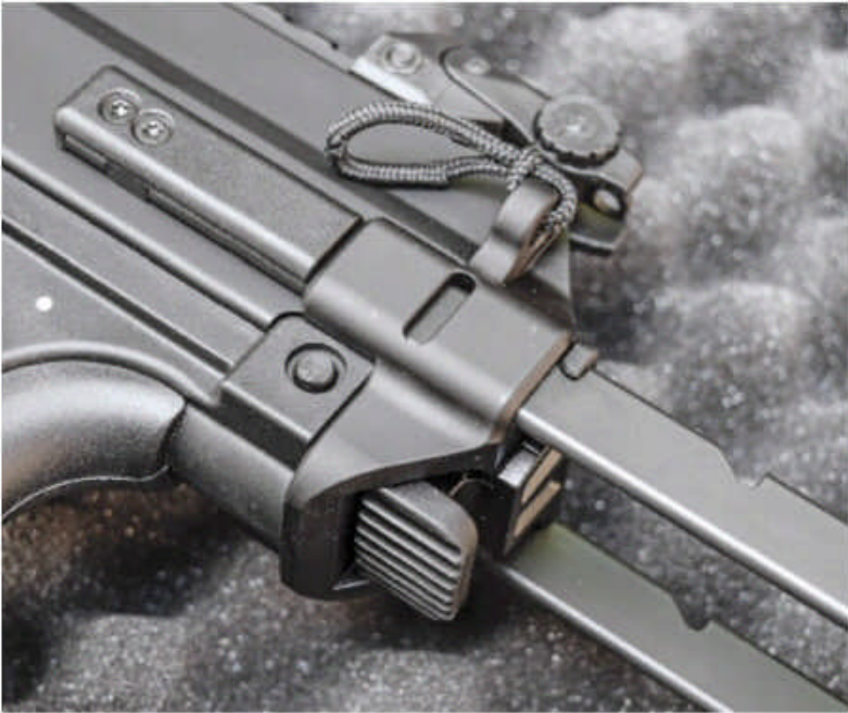
The collapsible brace adapter uses the same arms as the stock, but has been modified so it does not extend as far, to keep the ATF happy. To extend it, just pull. To close it, push up on the big button seen here.
