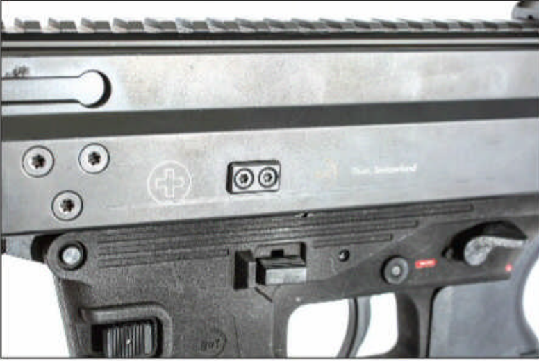
The upper is an aluminum tube, machined for the bolt, and with the barrel, ejector and other parts attached.
