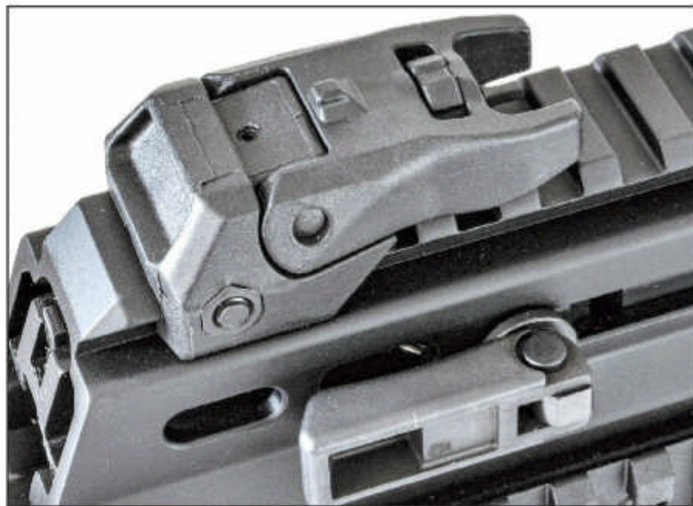
You can see how flat the charging handle folds. Check out the nub in the center of the folded front sight—that is a crude front sight post that can be used through the optic when the sights are folded.
