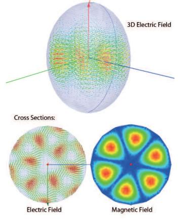
Figure 1: An electromagnetic resonant mode forming in a three-dimensional dielectric ellipsoid is a three-dimensional pattern of energy consisting of unique electric and magnetic field components. Here red shows the highest field strength and blue the lowest.
