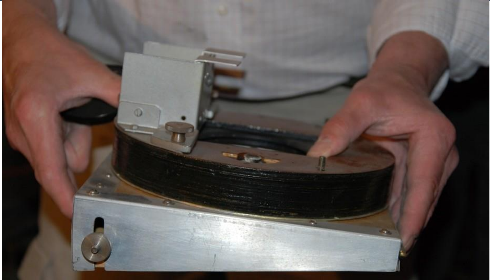
Adrian Kutter showing the plate adapter for the tilted field of the 300 mm Kutter telescope.
