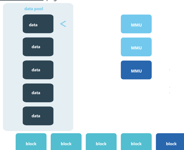
Figure 16. Adding Data to ESB. MMUs add data to the data pool for storage (dotted line) and pull data from the data pool (solid lines) and sign the resulting blocks (lower right). Signed blocks are appended to the global ESB.
