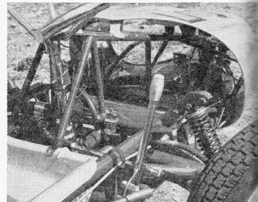
THE OFFICE: Direct "handlebar" steering, swing axle front suspension and gear lever connected with Norton "foot" change.
