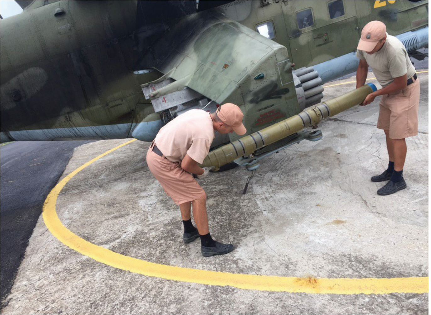
Armorers seen installing an 9M114 Shturm-V ATGM on the Mi-24P at Hmeimim.
