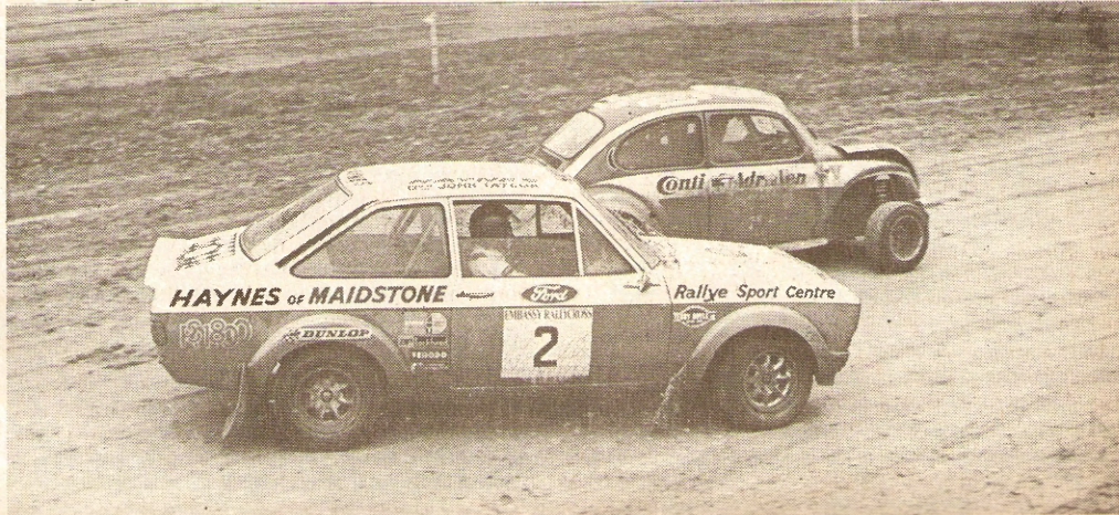
The slippery conditions just didn't suit cars with the drive and engine at opposite ends.
