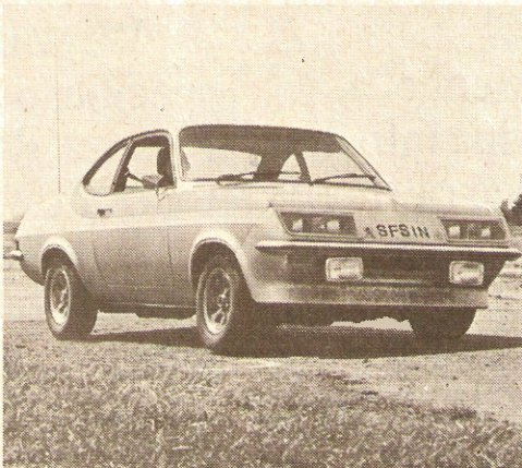
With 185 section tyres fitted, the rubberware graunches painfully on the body during hard cornering.
